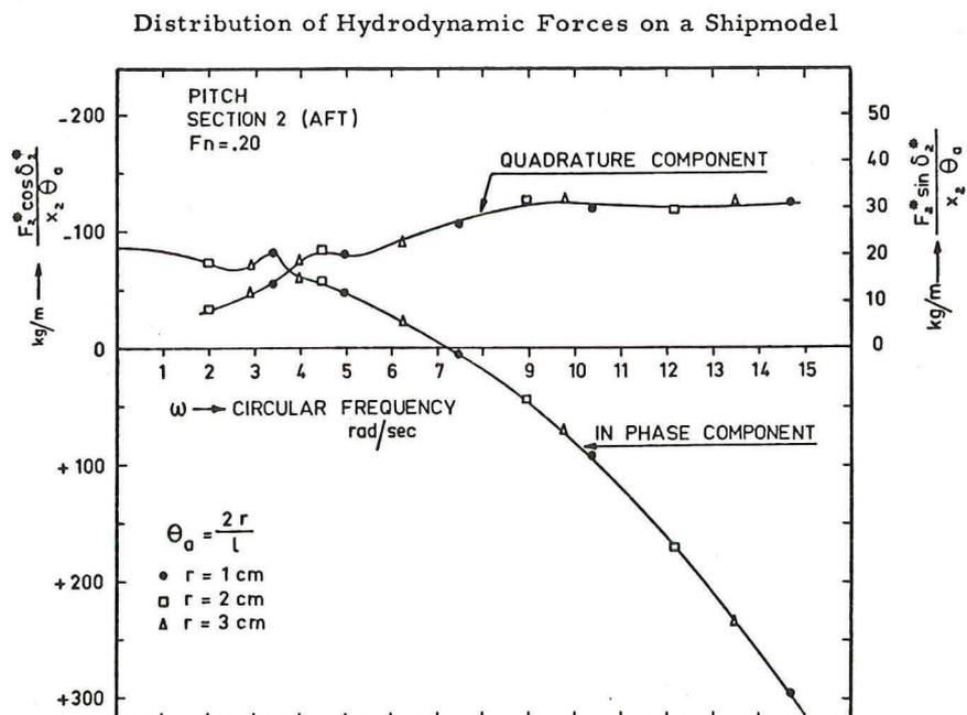
Fig. 4 - Components of force on section 2, pitching motion
