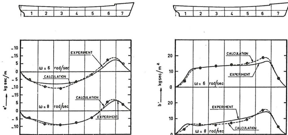
Fig. 14 - Comparison of the calculated distribution of  $e$  and  $b$  with experimental values for Froude number 0.20
