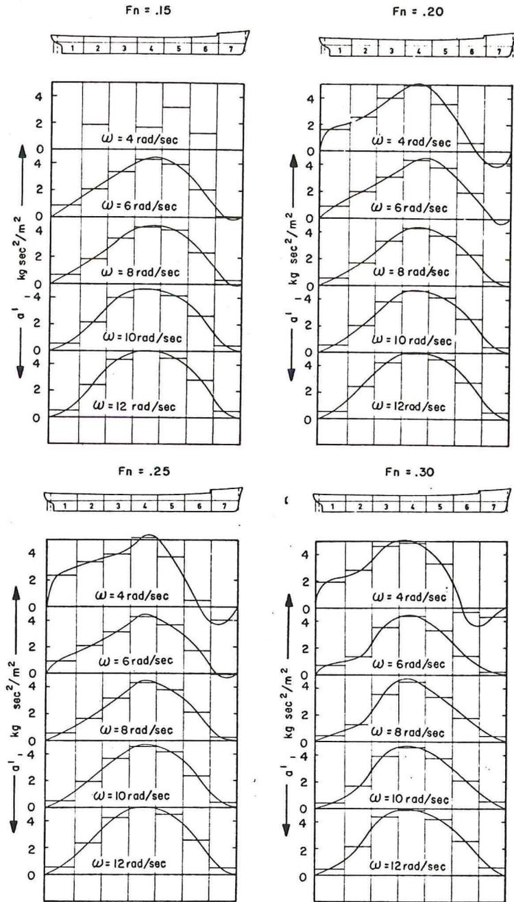
Fig. 7 - Distribution of  $a'$  over the length of the shipmodel
