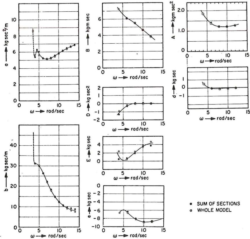
Fig. 11 - Comparison of the sums of section results and the whole model results for Froude number  $F_n = 0.20$
