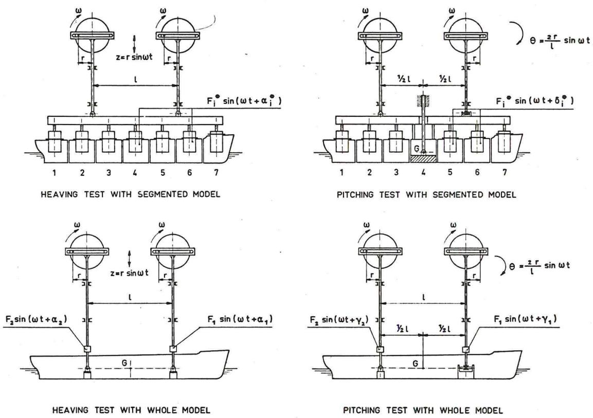
Fig. 2 - Arrangement of oscillation tests
