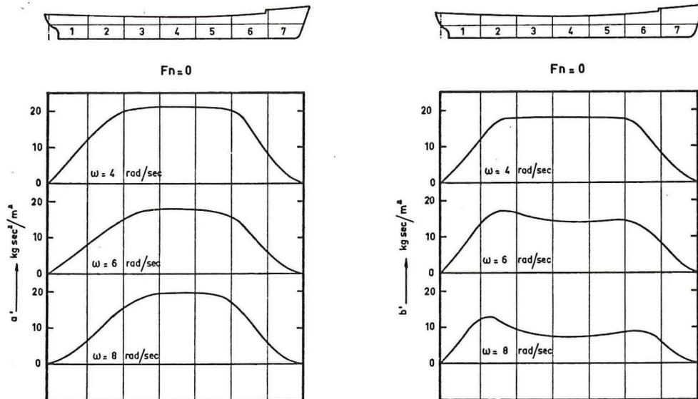
Fig. 12 - Calculated distribution of  $a$  and  $b$  for zero speed
