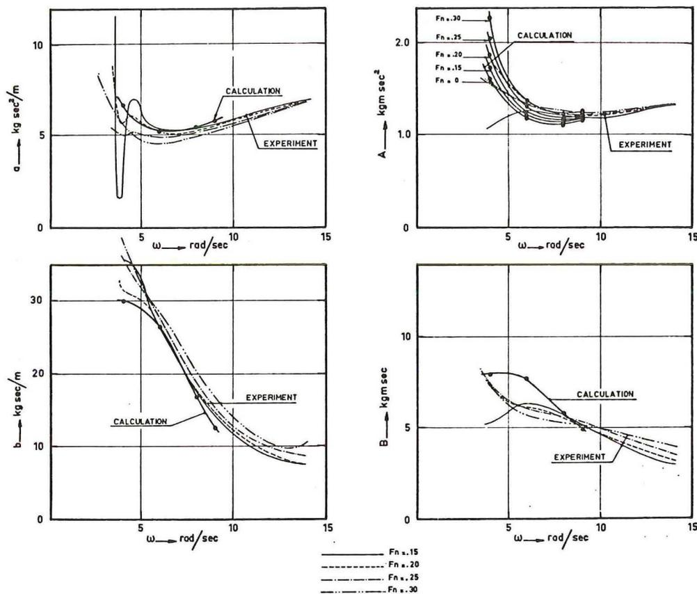
Fig. 15 - Comparison of calculated and measured values for  $a$ ,  $b$ ,  $A$  and  $B$  (whole model)
