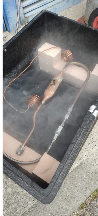
Figure 3.18: 20 bara high-pressure test under liquid nitrogen cooling.
