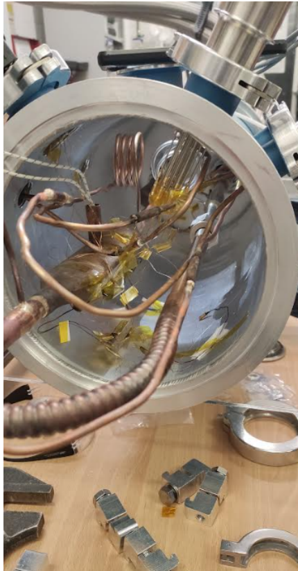
Figure 3.21: Image showing the CERNOX cryogenic temperature sensor and electrical heating mounting onto the heat sink.
