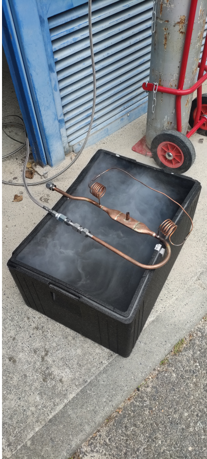
Figure 3.17: 20 bara high-pressure test under cold nitrogen vapor cooling.
