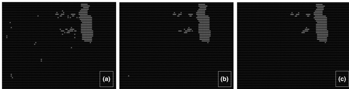
FIGURE A4 Graph illustrating the cleaning procedure of the cellular automaton algorithm using a set of rules (see text for more details) for the P10 case. Zeros correspond to “populated” cells and dots to “unpopulated” ones. Shape convergence in this example is achieved after two iterations. Initial and final states in (a) and (c), respectively
