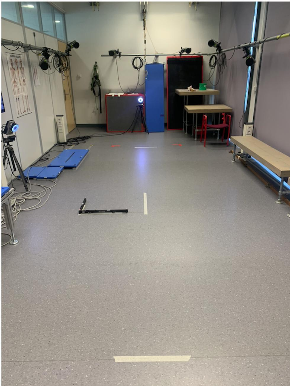
**Figure F.1:** Calibration setup of the Gait Lab of the faculty 3me at the TU Delft. The Qualysis L-frame on the ground serves as the local reference lab frame for this system.
