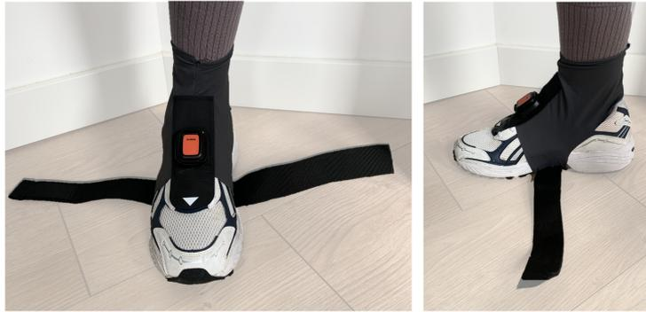
**Figure 5.1:** Sock Concept, for the sensor-to-shoe fixture with the fixation band open, front and side view respectively.
