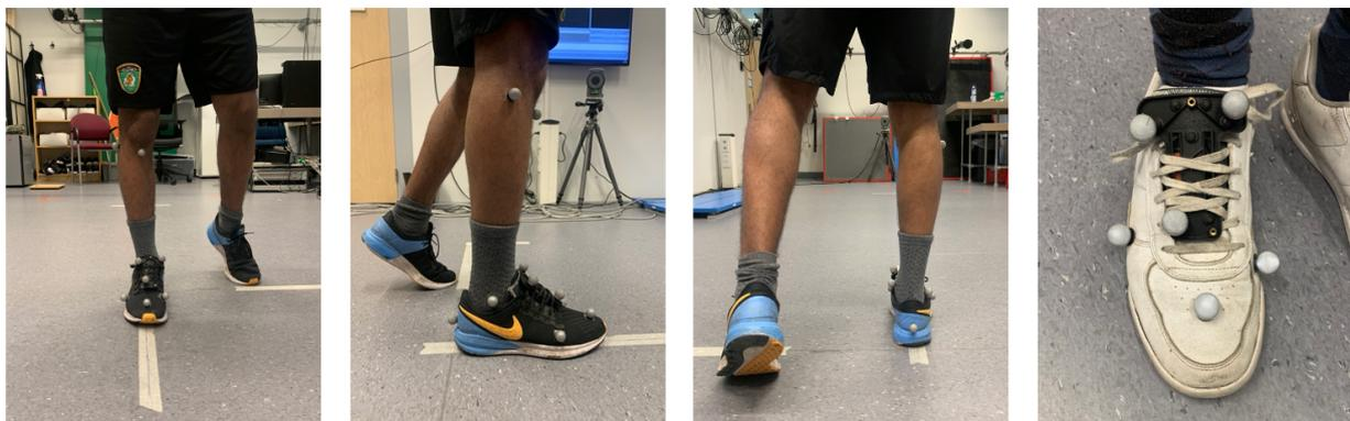
**Figure 7.1:** Marker Placement on one of the participants from front, side and back view. And a close-up of the marker placement on the foot of one of the participants, and the sensor with the fixated marker cluster of Qualisys with markers located at positions 1, 3 and 4.
