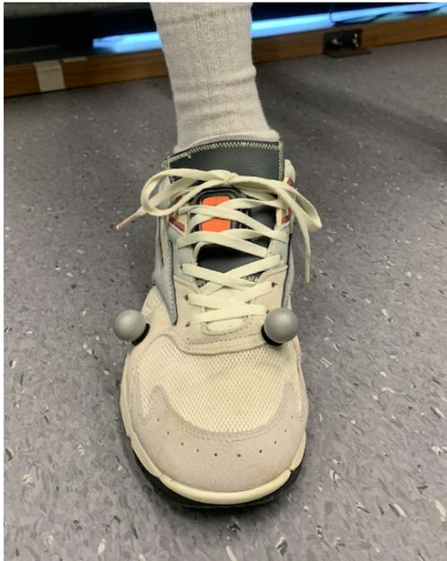
**Figure 11.1:** Participant P7's sensor-to-shoe fixture, showing incomplete alignment with the shoe tongue due to it being sewn to the shoe body, complicating the placement of the fixture.
