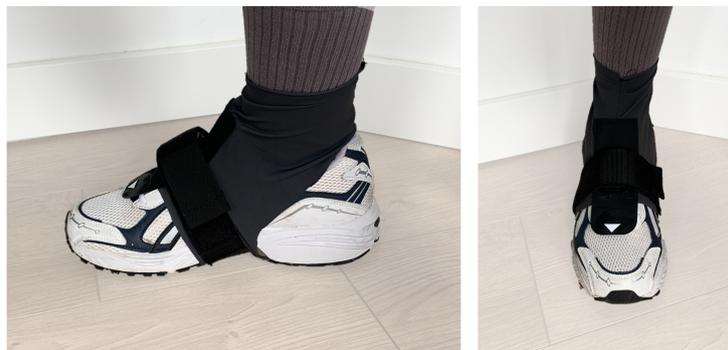
**Figure 5.2:** Sock Concept, for the sensor-to-shoe fixture with the fixation band open, side and front view respectively.
