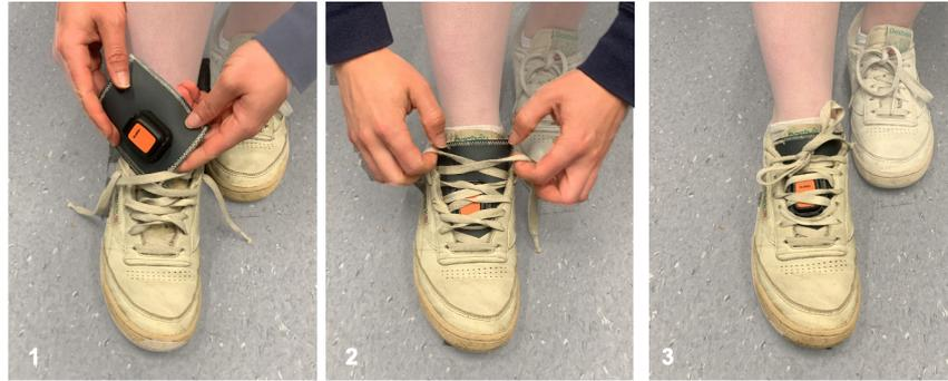
**Figure 5.3:** (1) Placing the sensor-to-shoe fixture on top of the shoe tongue underneath the laces. (2) Tighten the shoelaces for fixation of the shoe and the sensor-to-shoe fixture. (3) Fixture with the sensor fixated on the shoe.
