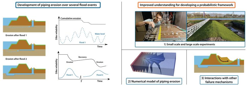
Figure 3: **Left:** Piping schemes adapted from <u>van Beek (2015)</u> and dike reliability graphs sketched by Joost Pol. **Right:** Main components of the research. Left photo © Sam Rentmeester and right photo and schemes by Joost Pol.
