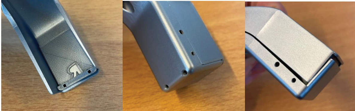
Figure 34 – Left to right: 3D printed part in the thumb part of the Hub, called the ‘gap closer’ among the employees; the gap closer pulls the shell halves together with screws inserted into the predrilled holes seen here; the issue the part is meant to prevent, external forces on the shell can cause a gap between the parts.
