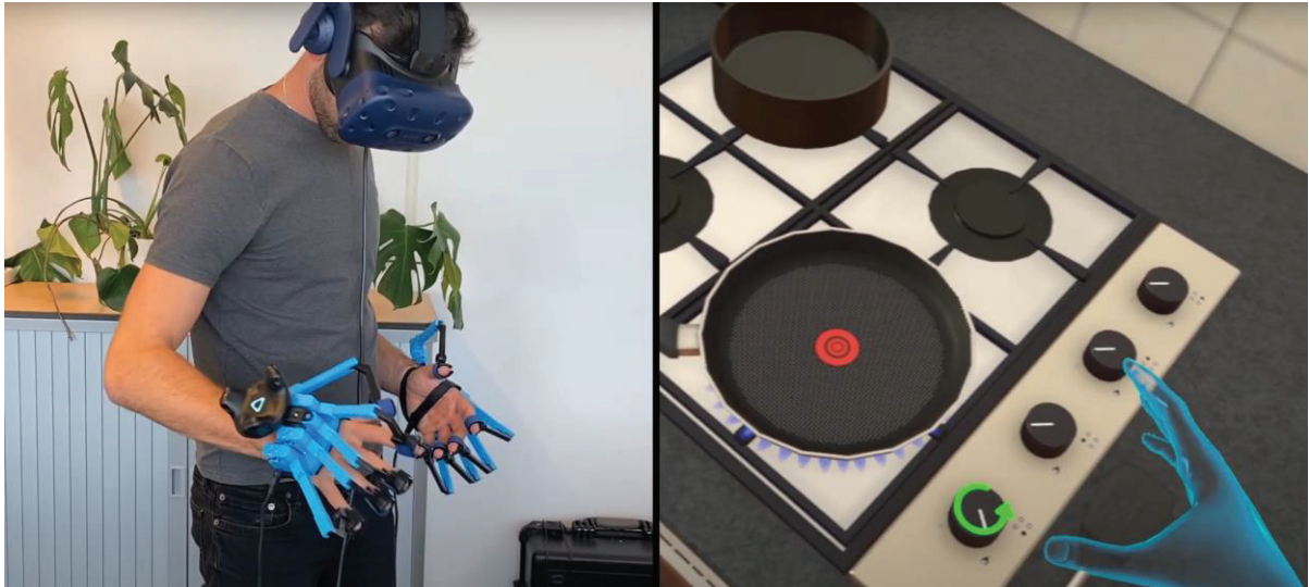
Figure 16 – Screenshot from video explaining SenseGlove's kitchen rehabilitation demo. On the left, we see the trainee interacting with DK1, Nova's predecessor. On the right, we see what the trainee sees.
