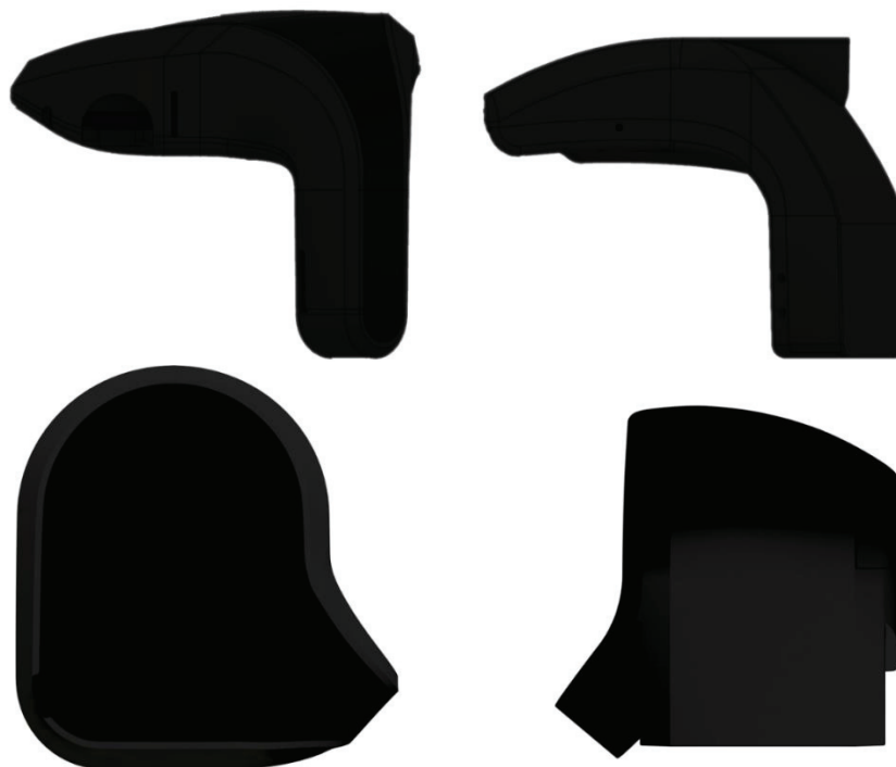
Figure 61 – Nova 2.0 and 1.0 silhouettes. In line with the aesthetic direction, the overall shape of Nova 2.0 has been kept simple and still mostly rectangular, with curvature in the corners instead of the sharp original shape.
