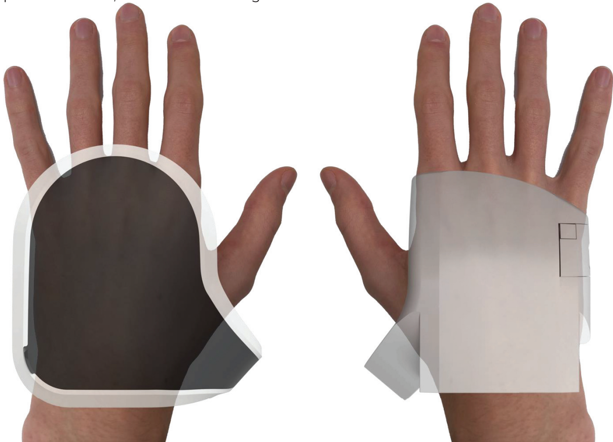
Figure 59 – Comparison of how Nova 2.0 overlaps the knuckles versus Nova 1.0. The increased length of the Hub is the result of new internal components and the rounded front as dictated by the aesthetic direction.
