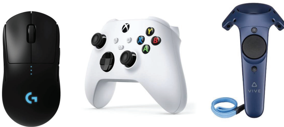
Figure 63 – Many input devices use an ABS shell for its desirable properties and price. Left to right: Logitech G PRO mouse, Microsoft XBOX One controller, HTC Vive Pro controller.
