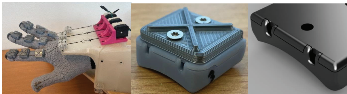
Figure 43 – Resin cable guides test showing that the cables can be guided without issues and without getting caught between the cable guide halves using special features at the end of each exit hole.
