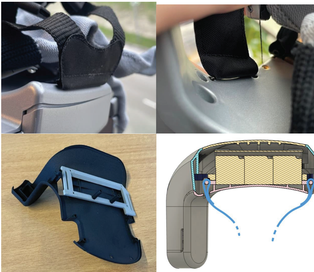
Figure 49 – Top: Original strap connection using threaded Nylon cables tied together inside the shell. While this saves on internal space, it requires dexterity and time during assembly. Bottom: New strap connection concept, with a single component below the FF modules that has the strap preinstalled and is lowered through holes in the shell before being screwed in place. Besides being easier to do, this method could also increase the strap connection's durability.
