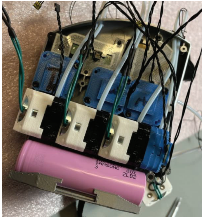
Figure 50 – Left-hand configuration of both stringpot (blue) and force feedback (white) modules inside Nova.
