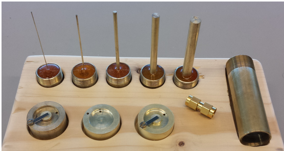
Figure 4.7: The realized coaxial impedance probe, note the different inner conductor diameters, as well as the different calibration terminations
