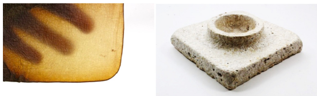
Fig. 1. Two examples of materials derived from living organisms. Left: thin, leather-like bacterial cellulose. Right: bulk mycelium composites.
