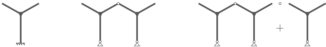
Figure 47 – Structural system to expand with more modules
