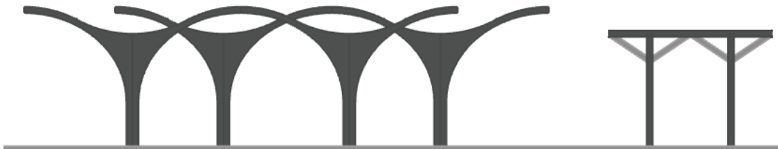
Figure 51 – Two side views show the shape and the stability system in two directions
