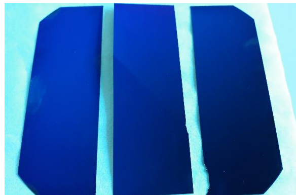
Figure 6: Three poor cut pieces, The left has become dirty due to improper handling, the middle one has a nick through it and the right one has a rough edge.
