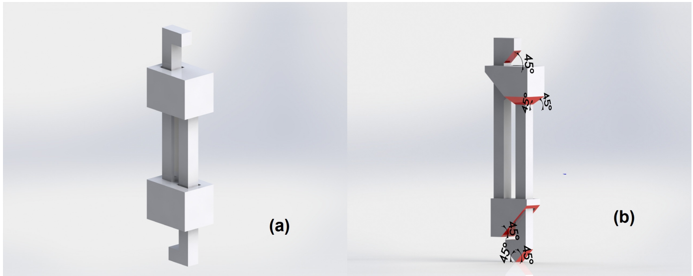
Figure 2.2: Illustration of a prismatic joint (a) and of a modified prismatic joint with inclined edges at an angle of 45^\circ (b).
