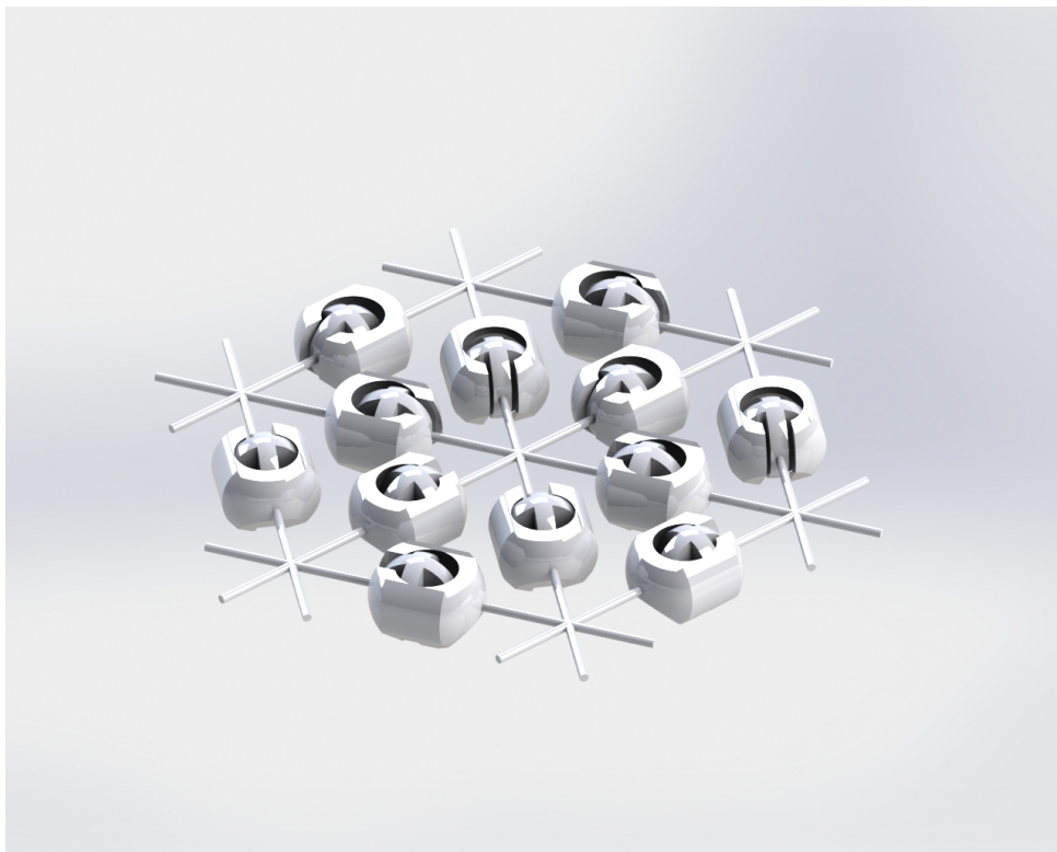
Figure 2.17: Star-shape configuration of multiple ball-socket joints.
