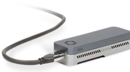
**Figure 1.3** USB-powered MinION™ sequencer
