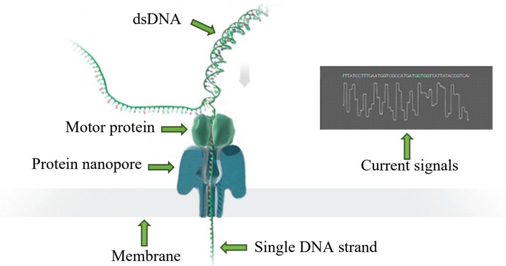
**Figure 1.1 Schematic representation of Oxford Nanopore DNA sequencing technology**
