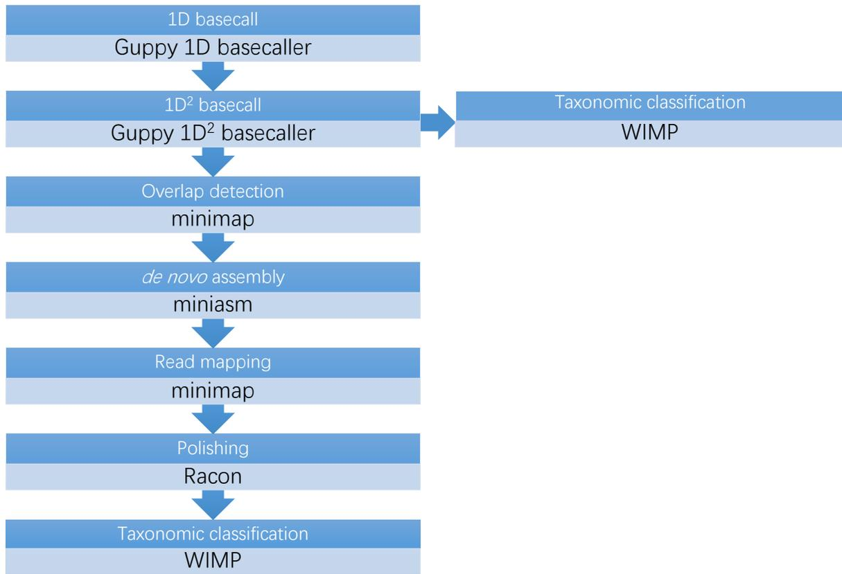
**Figure 2.3 Bioinformatics pipeline for processing MinION™ genomic DNA sequencing data**
