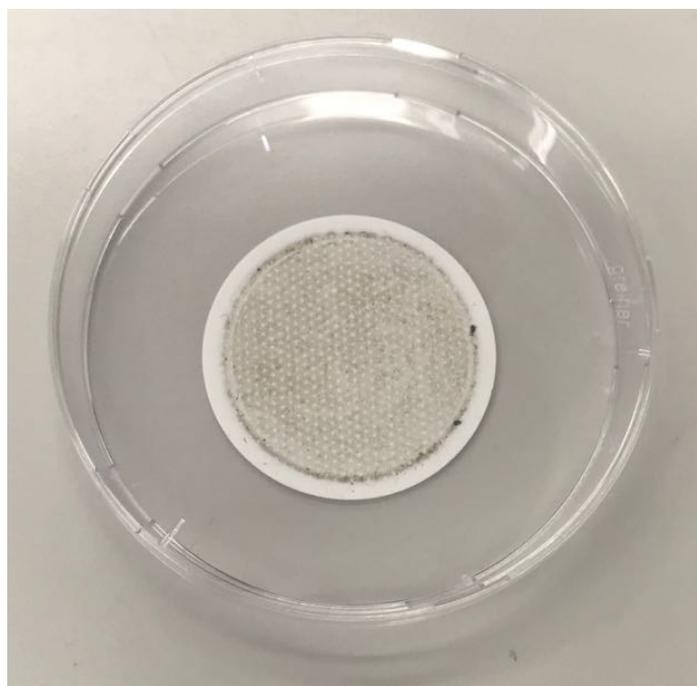
**Figure 3.1** Petri dish with a used PES filter membrane
