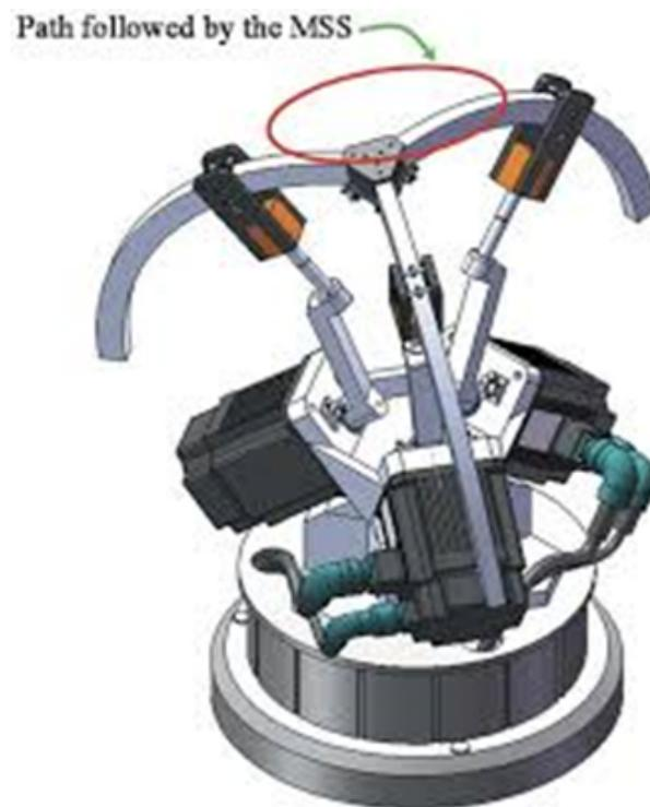
Figure C.13: A 3RRcP (circular track for prism), allowing for rotational movement [30]
