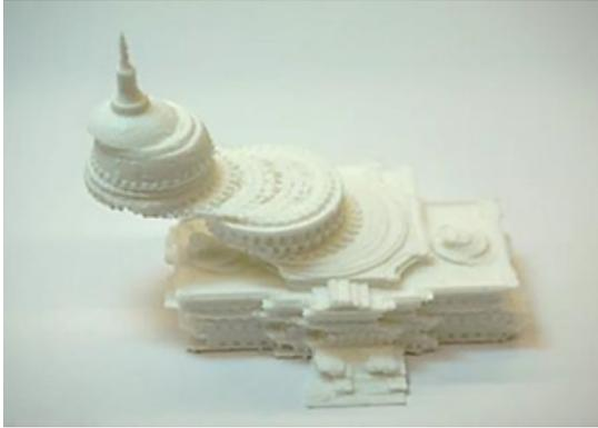
Fig. 16: Layers of FDM print shifting [88]
