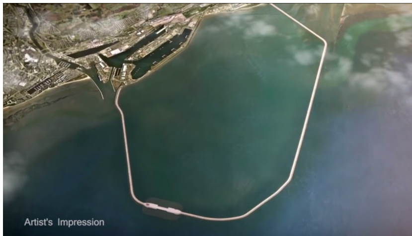
Figure 1.4: An artist's impression of the Swansea Bay Tidal Lagoon next to the city harbour. The turbines are located at the wider section at the bottom. Image from "Tidal Lagoon Power" [b]
