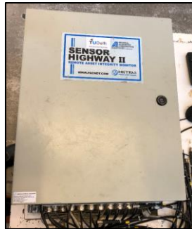
Figure 15 – Sensor Highway III data acquisition system
