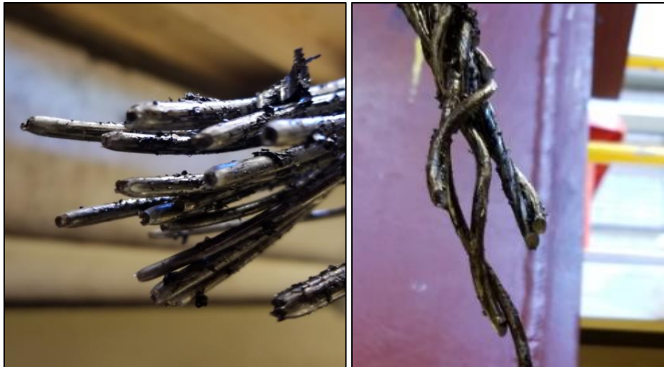
Figure 25 – Cup and cone failure (l) and shear failure (r)
