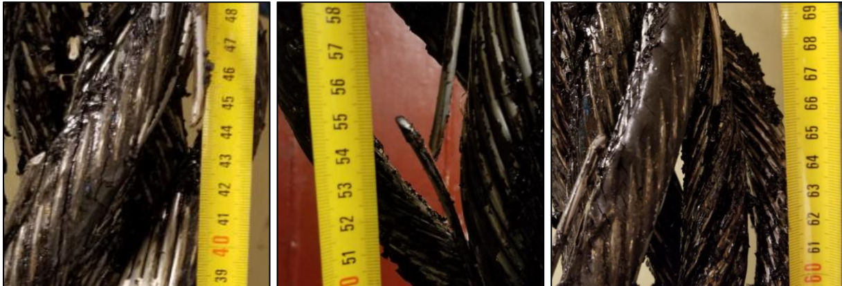
Figure 38 – Locations of clearly visible wire breaks
