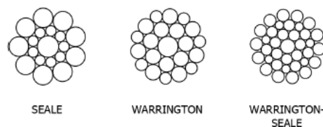
Figure 42 – Mostly used strand configurations (Ivanov, 2018)
