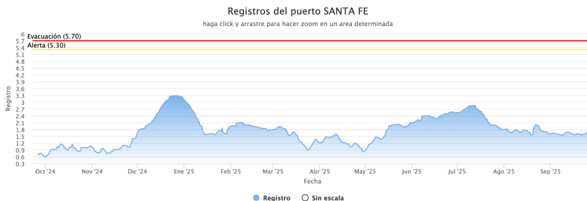
Figure 3.2: graph of hydrometric measurements Port of Santa Fe
