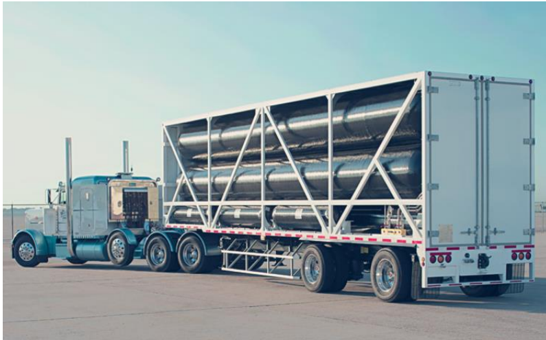
Figure 31; Mobile hydrogen container (Hexaconlincoln, 2019)
