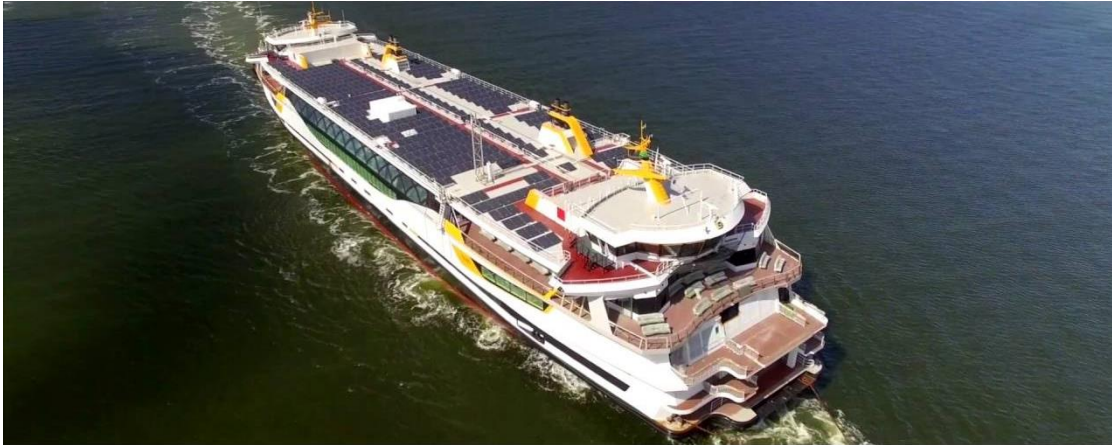
Figure 29; Solar panels placed on top deck of MS Texelstroom (C-Job, 2019)
