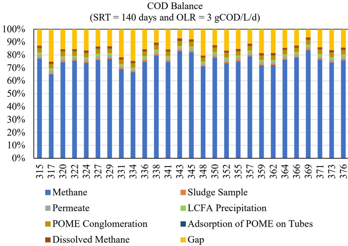
*Figure 14. COD Balance during Phase I*
