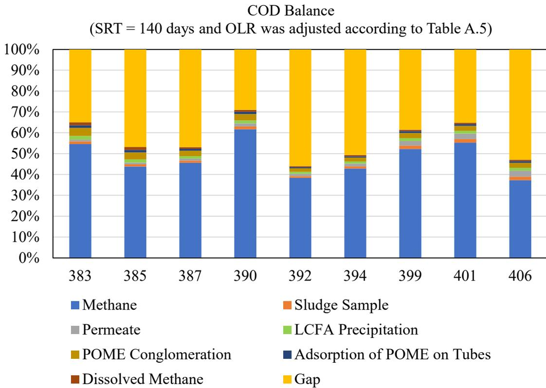
*Figure 15. COD Balance during Phase II*
