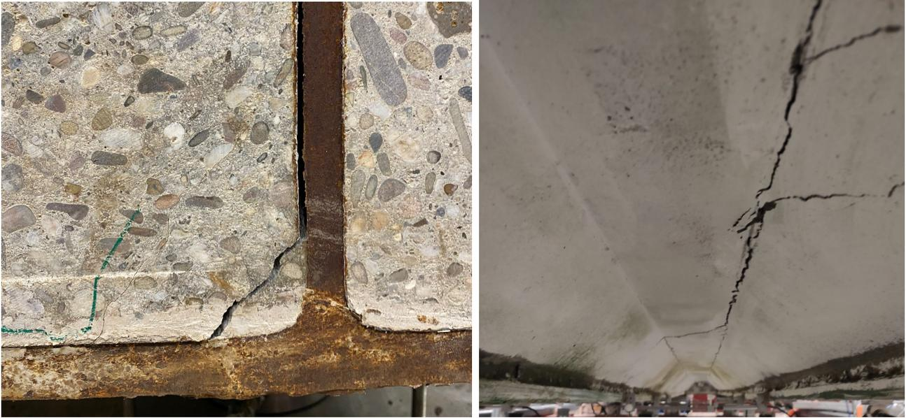
Figure 3.16: At the left: Opening between steel and concrete at one of the exterior girders observed after the failure of LB1. At the right: Longitudinal cracking observed after the failure of LB1.[34]
