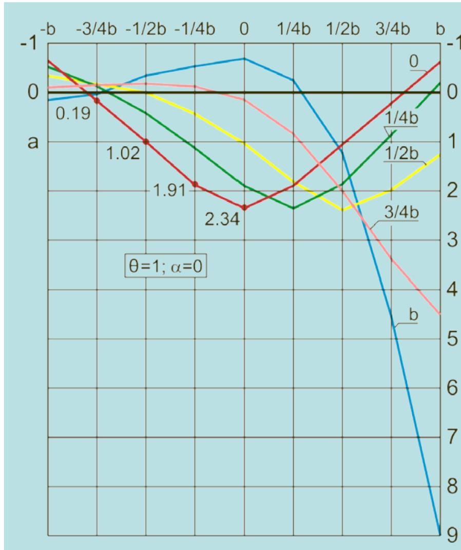
Figure 2.16: Influence lines at reference points between 0 and b [31].
