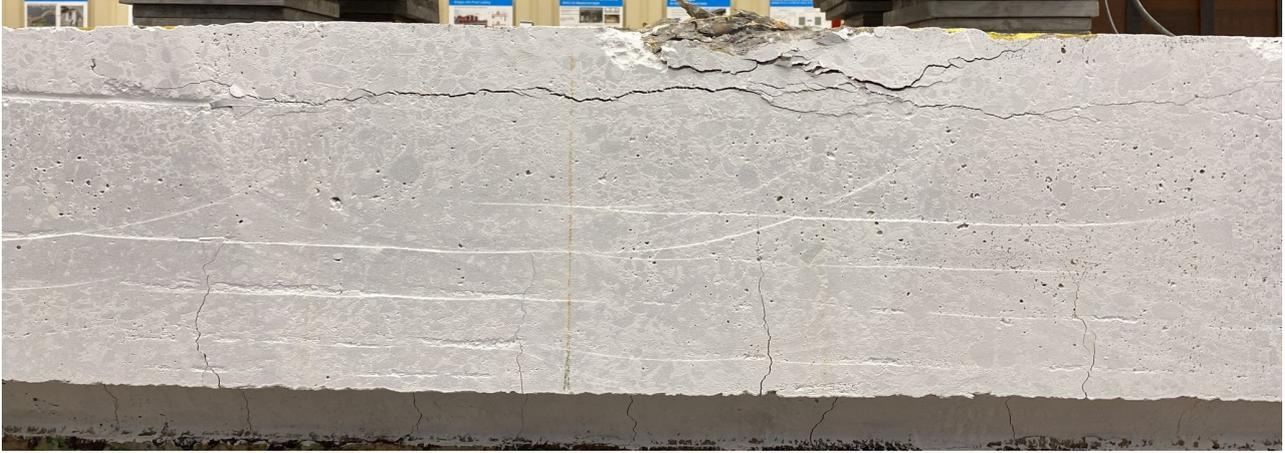
Figure 3.18: Sideview of LB3 showing concrete crushing at the top concrete fibre following failure [34].
