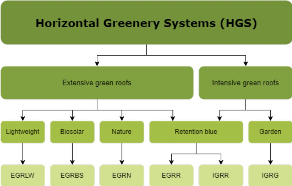
Figure 5.9: Overview of the Horizontal Greenery Systems that are considered in this thesis (own work)
