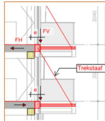
Figure 7.4: Balconies with tension rods in Urban Woods [52]
