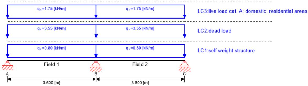
Section: CLT 160 L5s - 2; Material: C24 spruce ETA (2022); Service class: service class 1; Fire resistance class: R 120
