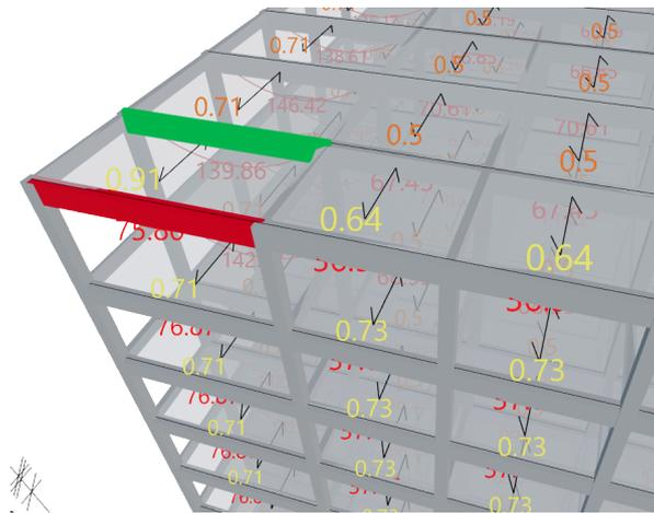
**Figure 11.6:** Unexpected unity checks for the concrete variant
