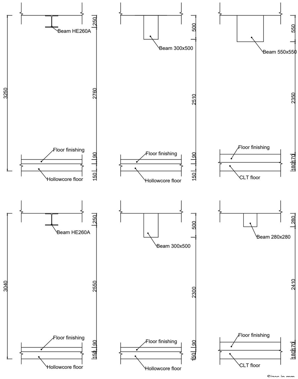
Figure 11.4: Check of the free height requirements for the different variants (left to right: steel, concrete, timber), for the top floor (top) and the lower floors (bottom) (own work)
