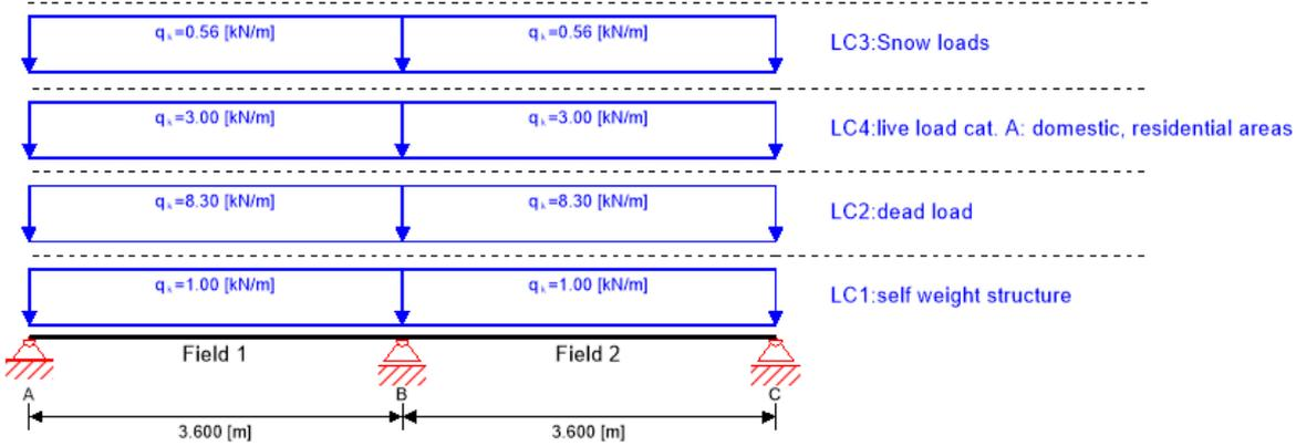
**Section:** CLT 200 L5s; **Material:** C24 spruce ETA (2022); **Service class:** service class 1; **Fire resistance class:** R 120
