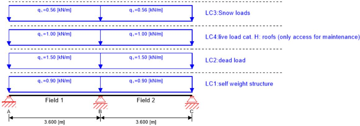
Section: CLT 180 L7s; Material: C24 spruce ETA (2022); Service class: service class 1; Fire resistance class: R 120
