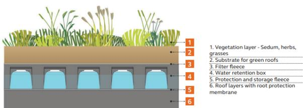
**Figure 5.7:** Extensive retention blue roof [57]
