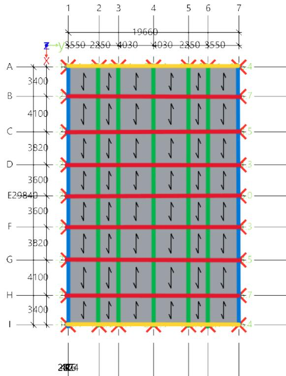
**Figure 8.4:** Primary internal beams (red), primary façade beams (yellow), secondary internal beams (green) and secondary façade beams (blue)
