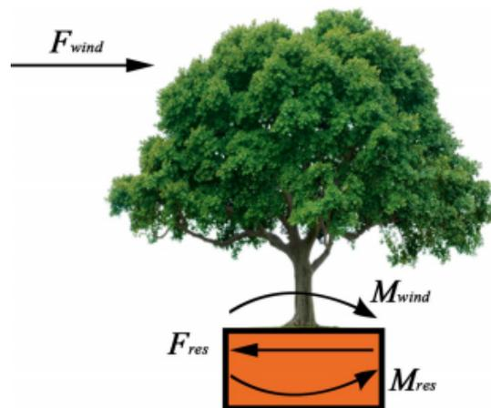
Figure 4.6: Loading conditions of a tree in a container [20]
