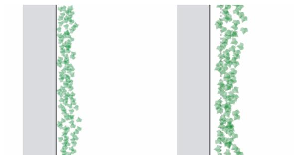
**Figure 6.1:** Green façade systems, from left to right: Direct Green Façade (DGF), Indirect Green Façade (IGF) [79]
