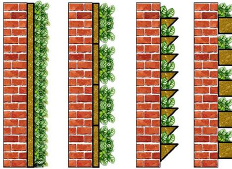
**Figure 6.2:** Living Wall Systems, from left to right: Continuous LWS (LWSC), LWS with Modular Boxes (LWSMB), LWS with Modular Trays (LWSMT), Linear LWS (LWSL) [86]
