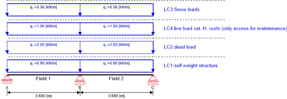
**Section:** CLT 180 L5s; **Material:** C24 spruce ETA (2022); **Service class:** service class 1; **Fire resistance class:** R 120
