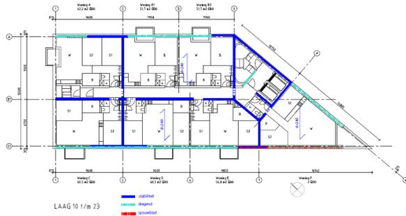
Figure 4.4: Spakler building construction of floors 10-23 [41]
