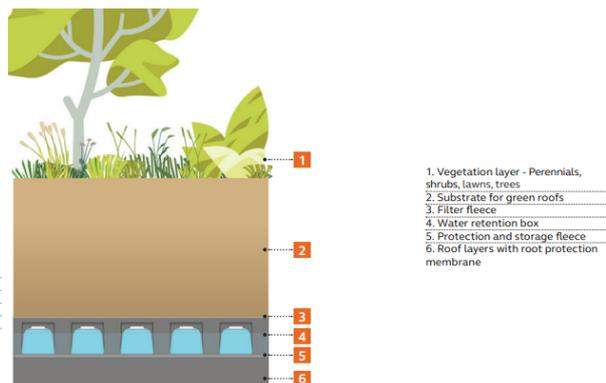
**Figure 5.8:** Intensive retention blue roof [57]
