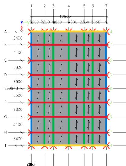
**Figure D.1:** Primary internal beams (red), primary façade beams (yellow), secondary internal beams (green) and secondary façade beams (blue)
