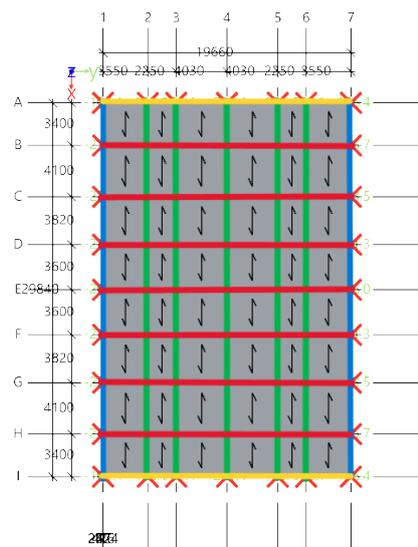
**Figure C.1:** Primary internal beams (red), primary façade beams (yellow), secondary internal beams (green) and secondary façade beams (blue)
