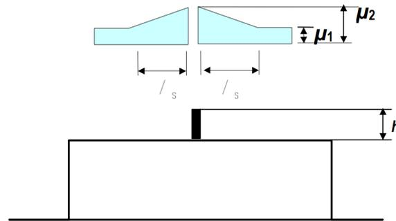
Figure 5.4: Snow accumulation coefficients at obstacles [64]
