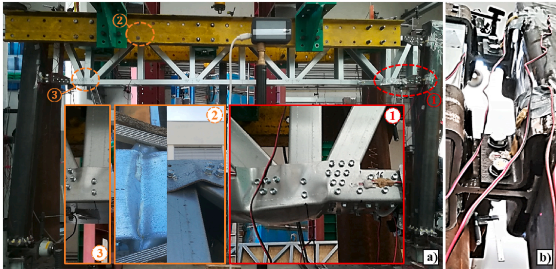
Fig. 15. Failure mode and post-test deformed configuration - FC2-H.
