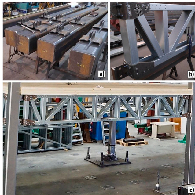
Fig. 1. The INNO3DJOINTS system: a) columns with the socket welded; b) truss-beam with the plug attached and c) the system post-assembly.
