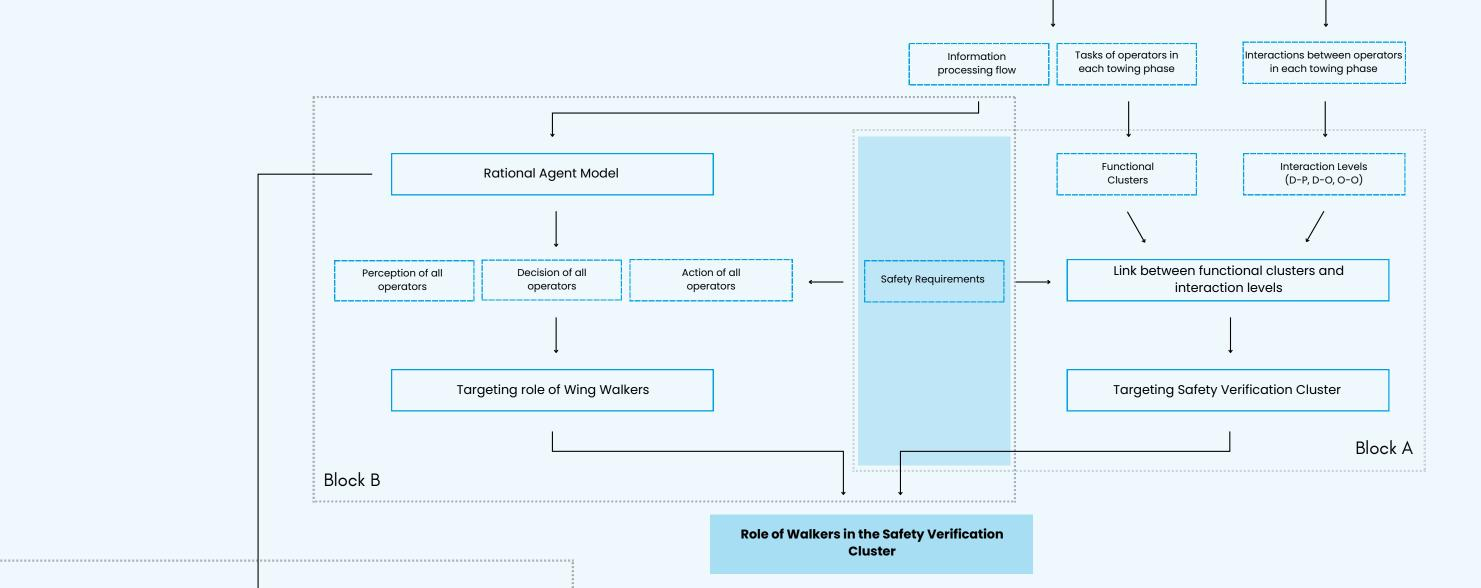
The framework indicates that a Level 2 perception system can replace the roles of the aircraft tail walker and wing walkers who provide insights to the driver while towing, ensuring the towing is performed safely.
