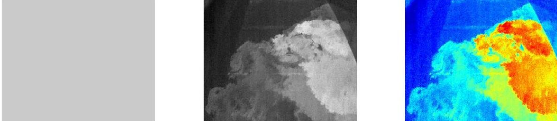
Figure 5. Plot of the frame. Full scale on the left, after temperature rescaling in the middle and after blue-red rescaling on the right. Discharge in the flume 100 l/s (15.9°C) and a lateral discharge of 2.84l/s (33.5°C) coming through the connection D 200mm.
