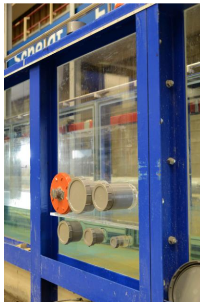
Figure 4. The experimental setup: photo of the diameter windows set up on the right bank of the Eastern Scheldt flume.
