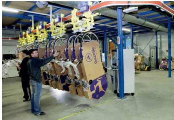
Figure 2.9: Damage reduction by storing the bicycles on the front wheel [7]
