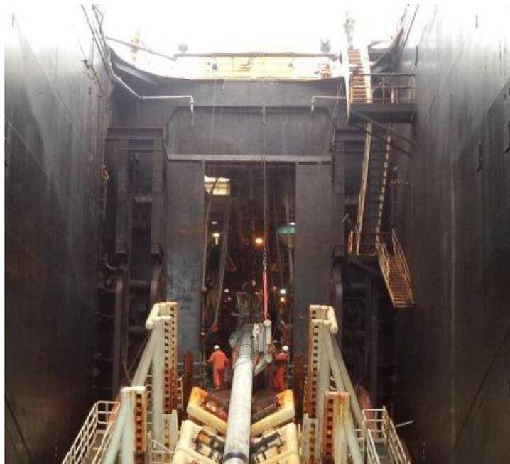
Figure 7.14: Stinger slot and possible location for the extra station. ©Allseas B.V
