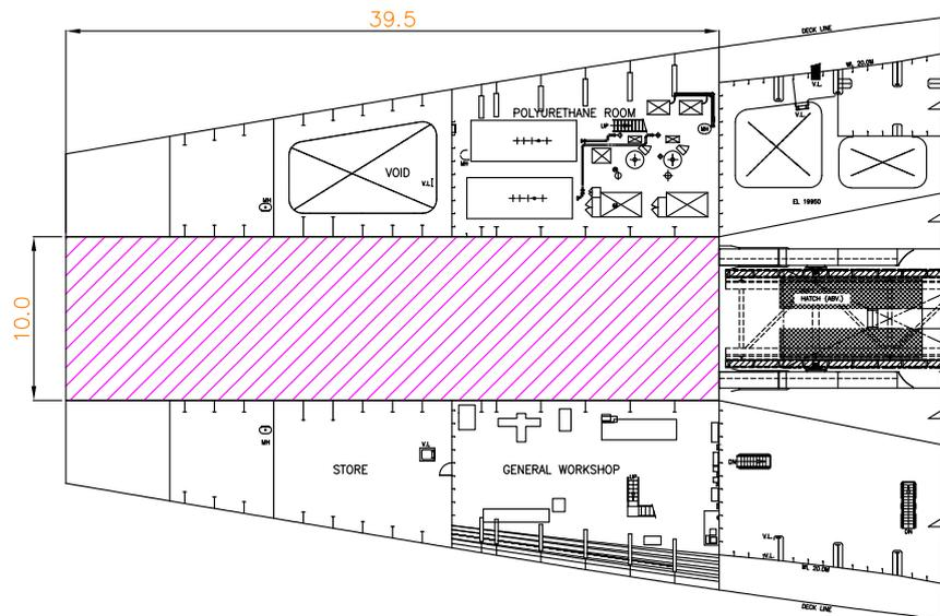
Figure 5.2: Possible extra deck space to extend firing line.
