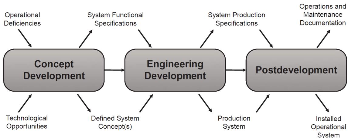
Figure 3.2: Main stages in a systems life cycle , from [2]
