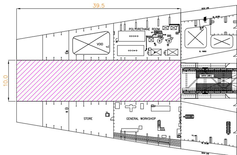
Figure 7.8: Plan view of Stinger Slot
