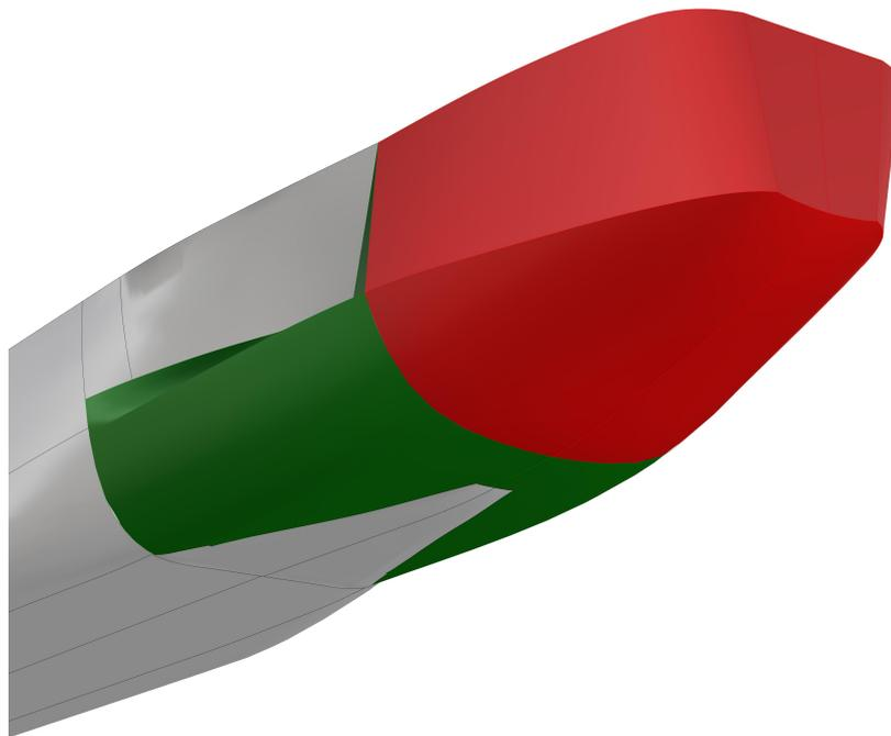
Figure 8.1.1: New aft hull forms. New structure in red, new shaped sponsons in green and Old structure in grey
