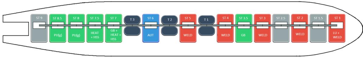
Figure 2.1: Schematic of firing line configuration for Nord Stream II. ©Allseas B.V
