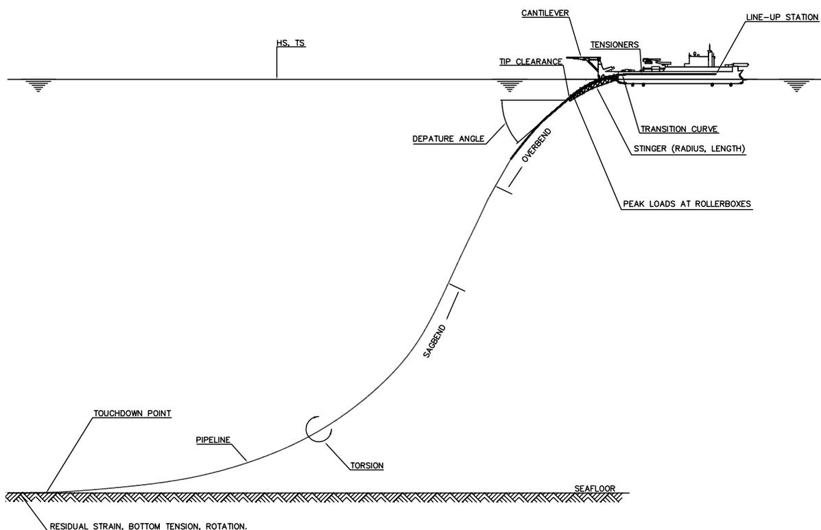
Figure 2.4: Schematic of S-lay. Adapted from [1]
