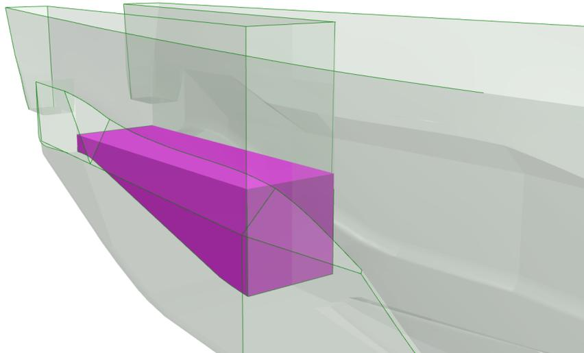
Figure 7.6: Added volume due to stinger slot closure
