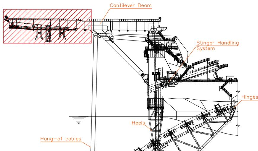
Figure 7.2: Removed part of the cantilever beam
