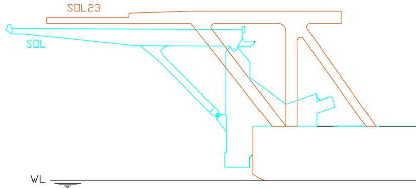
Figure 8.5.2: Aft lateral area (above water) comparison.
