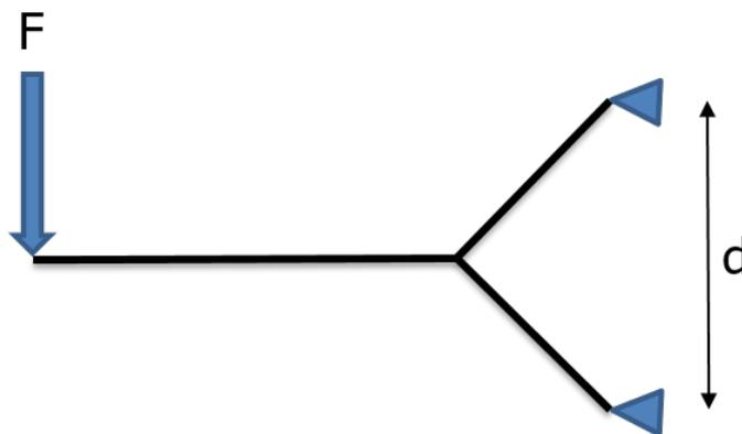
Figure 5.1: Free body diagram model of stinger
