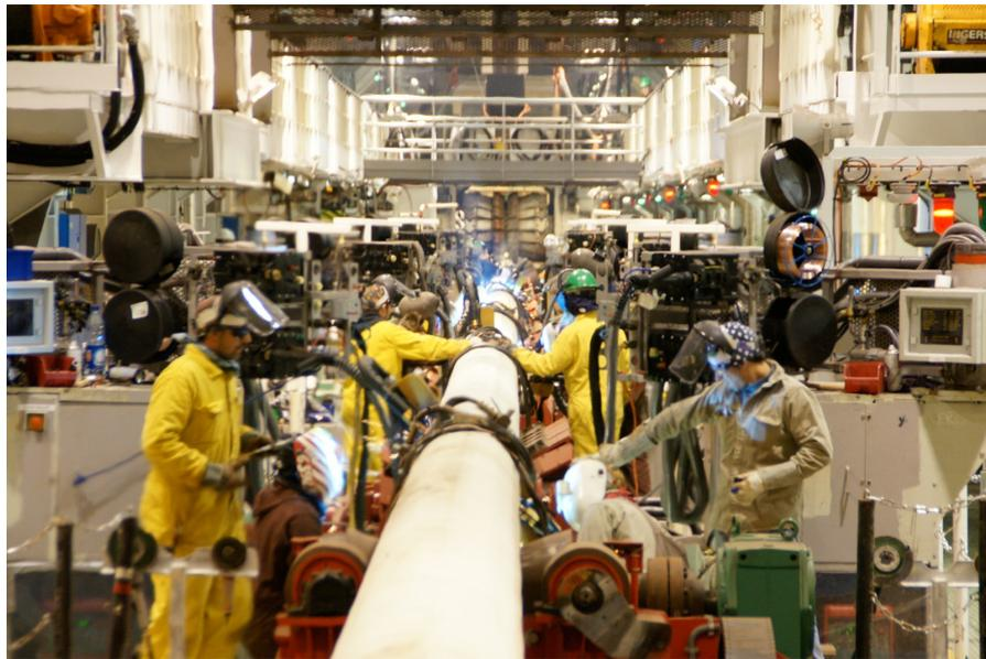
Figure 2.2: Firing line. ©Allseas B.V
