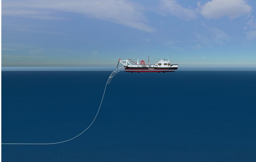
Figure 2.3: S-lay diagram. ©Allseas B.V
