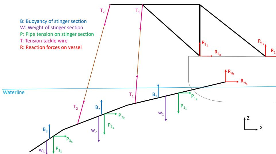
Figure 8.3.1: Free-body diagram of Stinger and SHF
