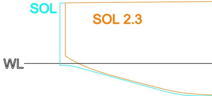
Figure 8.5.1: Aft lateral area comparison
