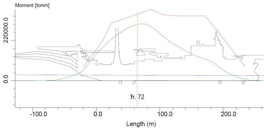
Figure 7.7: Bending moments LC 20 with stinger slot closed
