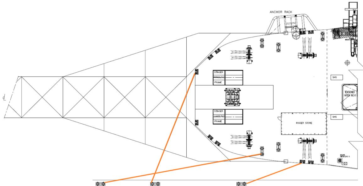
Figure 8.2.2: Example of aft mooring lines to quay side
