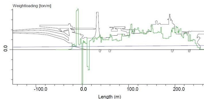
Figure 8.3.2: New weight distribution of loading condition "Arrival ballast"
