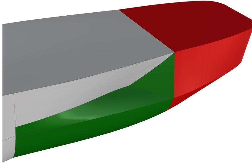
Figure 8.1.2: Top view of new aft hull forms. New structure in red, new shaped sponsons in green and Old structure in grey
