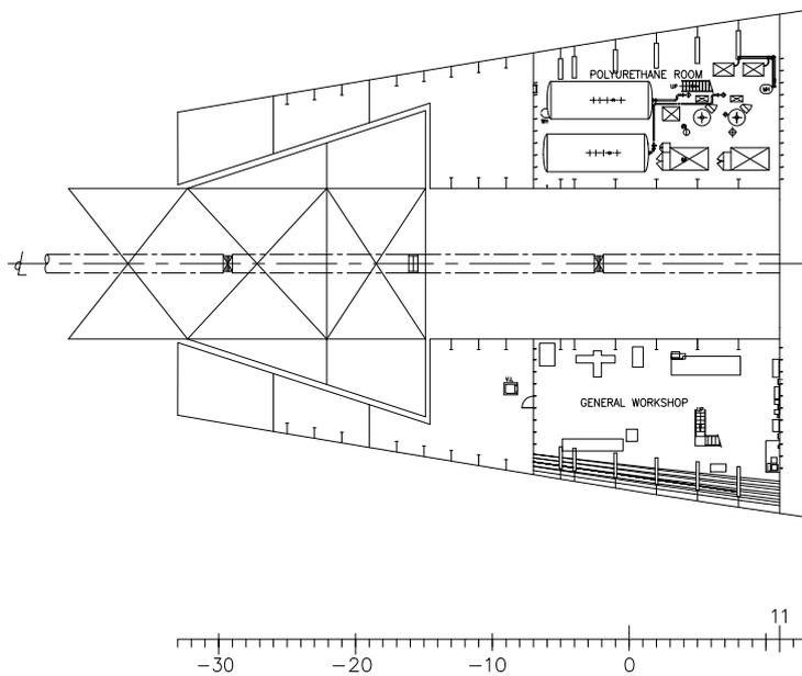
Figure 7.10: Sketch of possible inside hinge stinger configuration
