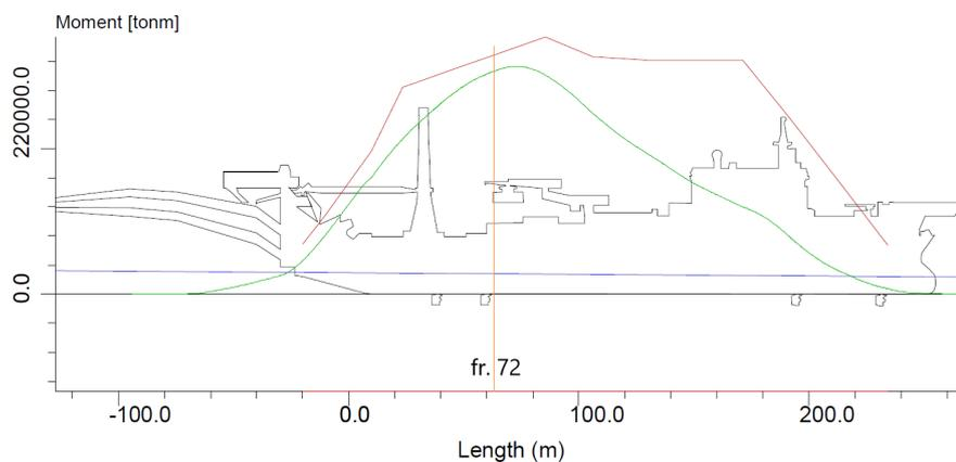
Figure 7.3: Bending moments LC 20 with modified cantilever beam
