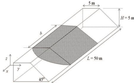
**Figure 1.** Failure mass within a 3D slope (based on Vanmarcke (1977)).
