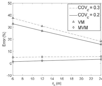
Figure 5. Error in mean 3D FS by VM and MVM with respect to mean 3D FS by RFEM
