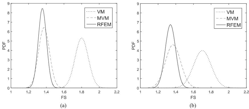
Figure 4. PDF of 3D FS obtained by the 3 methods for: (a)  $\theta_h = 6$  m and (b)  $\theta_h = 12$  m.
