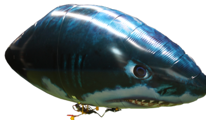
Figure 7.2: Blimp's Microfoil envelope with the gondola attached.
