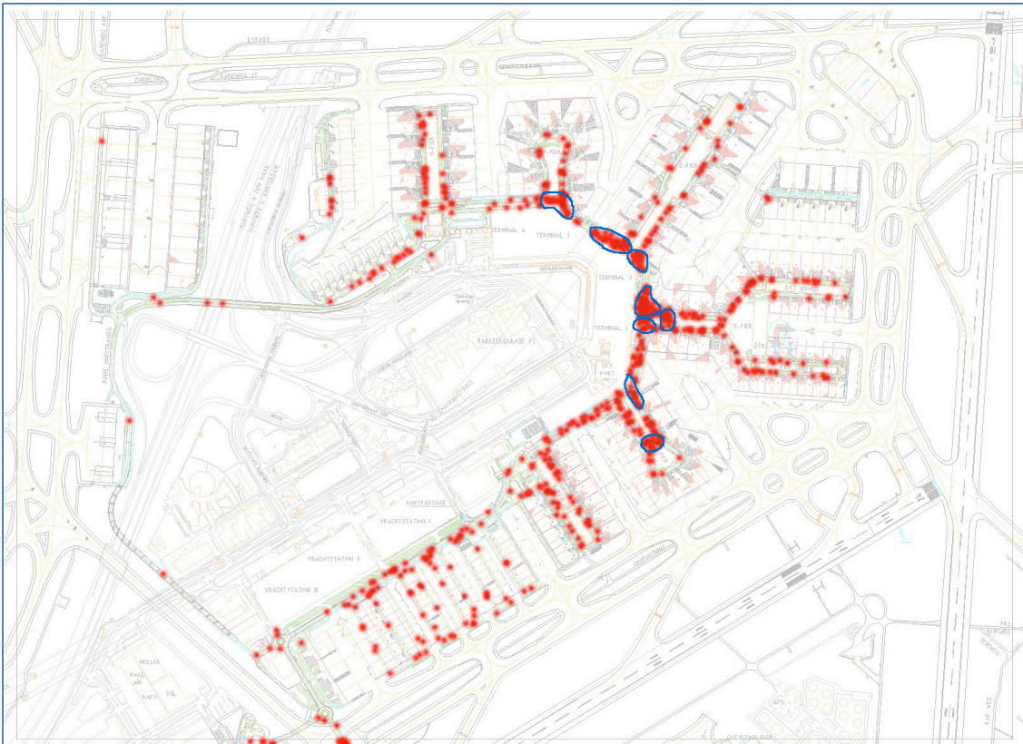
Figure 3.19; Problem areas of collisions between vehicles
