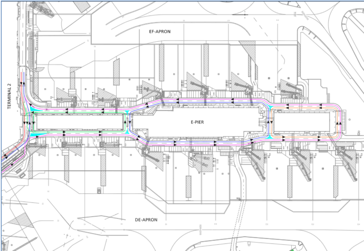
Figure 7.3; Proposed improvement possibility for changing the E-pier in a complete one-directional situation (Verhaar, 2012)
