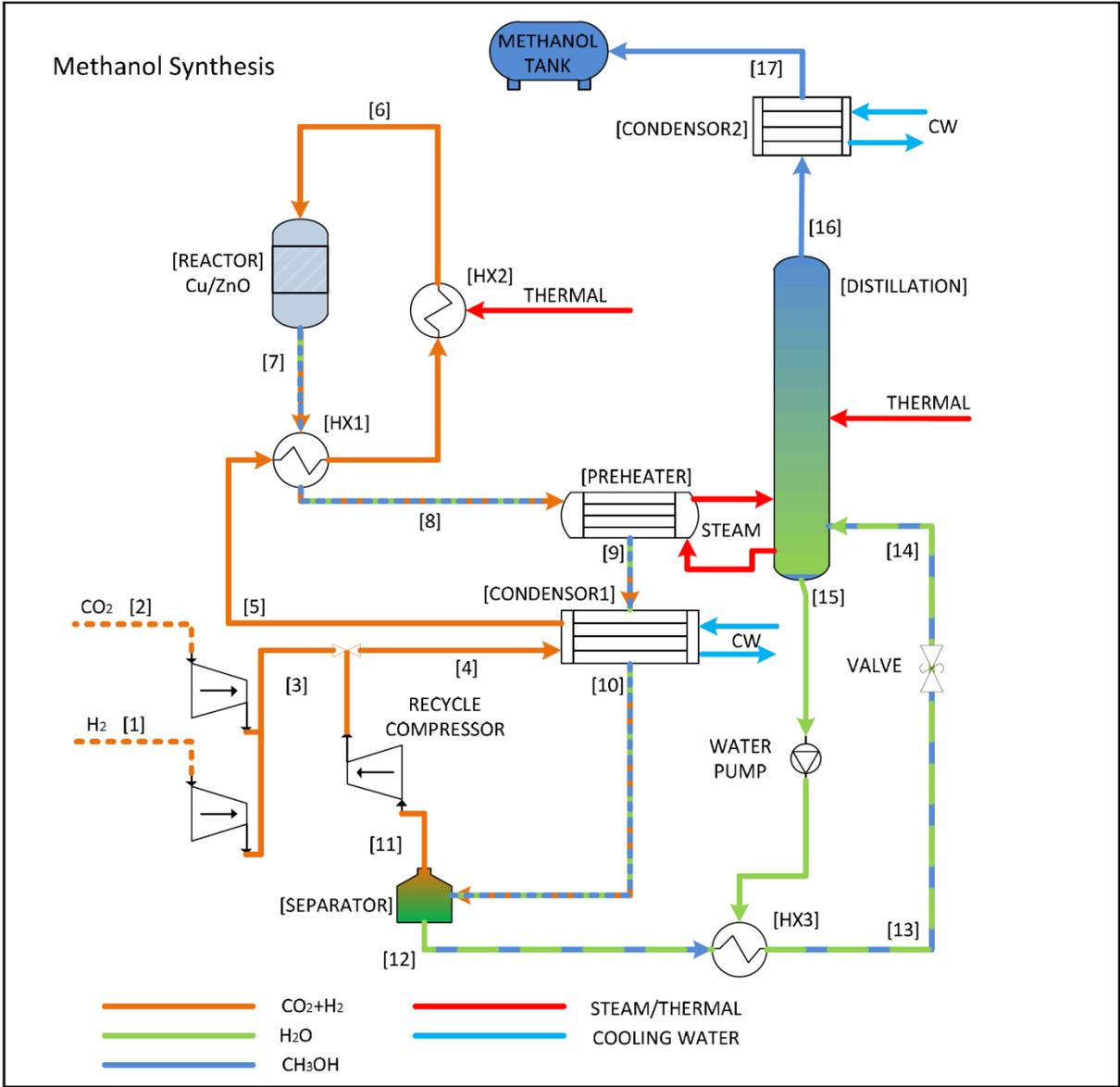
Figure 1 – Lurgi Methanol process parameters (Kauw, 2012)
