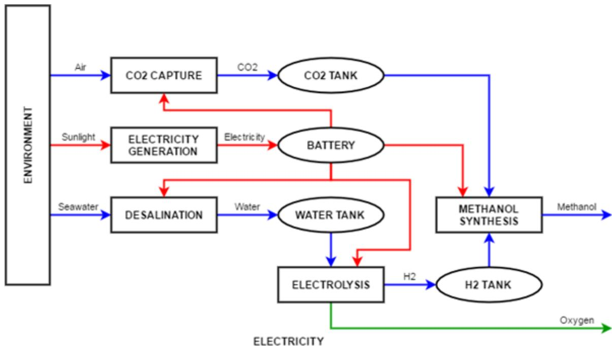
Figure 4 – Flowchart representation of the process in the COS
