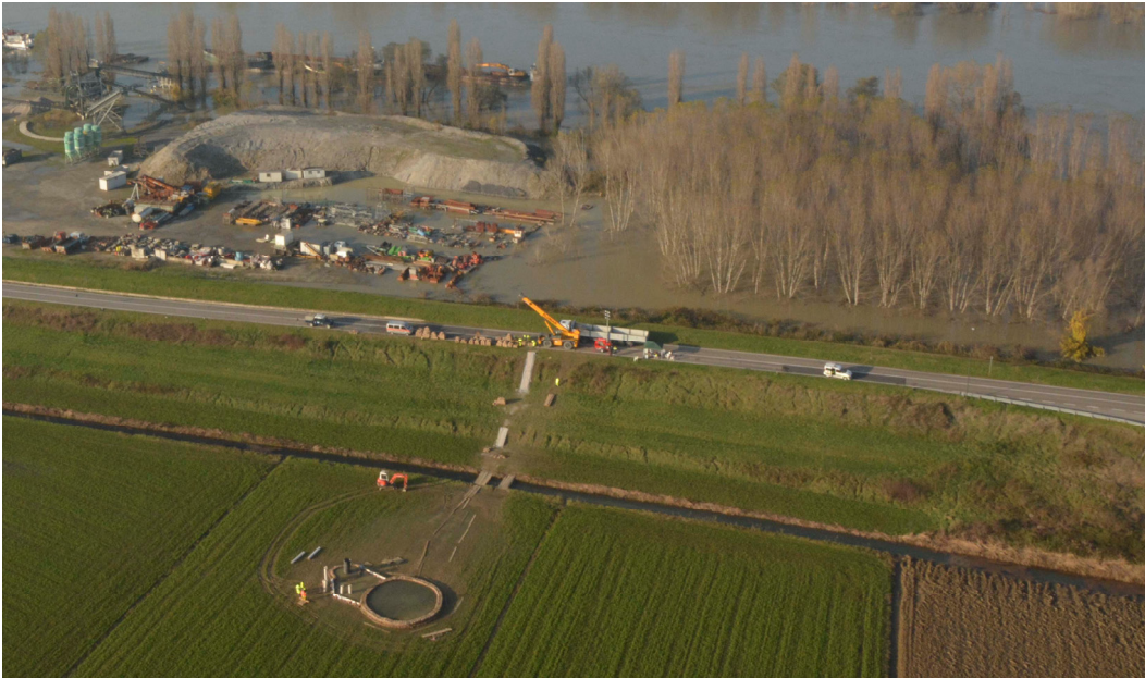
Figure 3. Ringed sand volcano near Boretto (Courtesy of AiPo).
