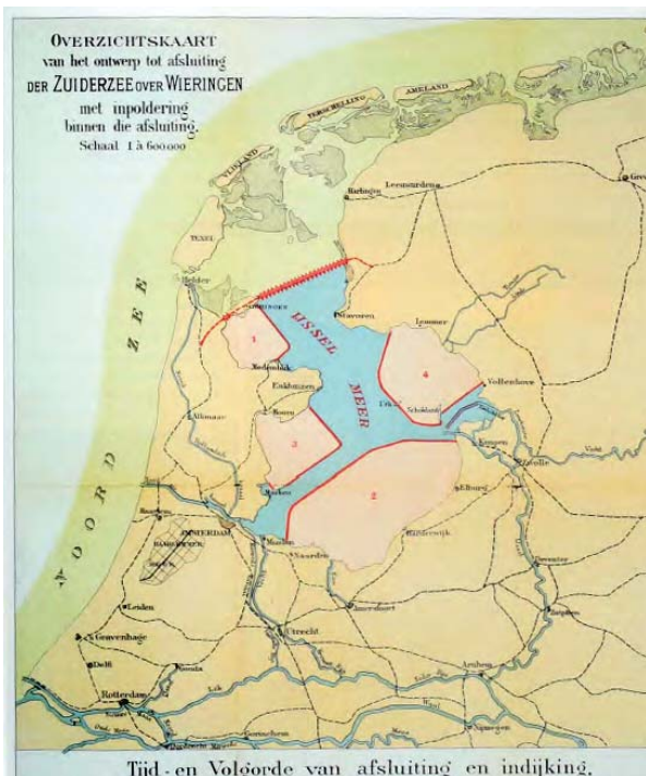
Figure 1.3 Map of the design for closing off the Zuider Zee, including the order and the time scheme for closure and construction, demonstrating strategic planning in 1901. Source: Mastering the City ||
