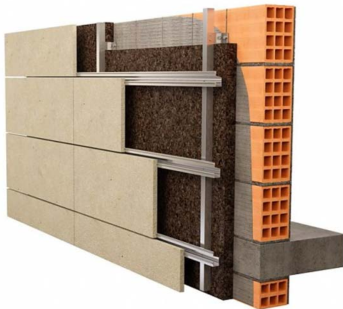
Figure 46: Ventilated facade with cork insulation
