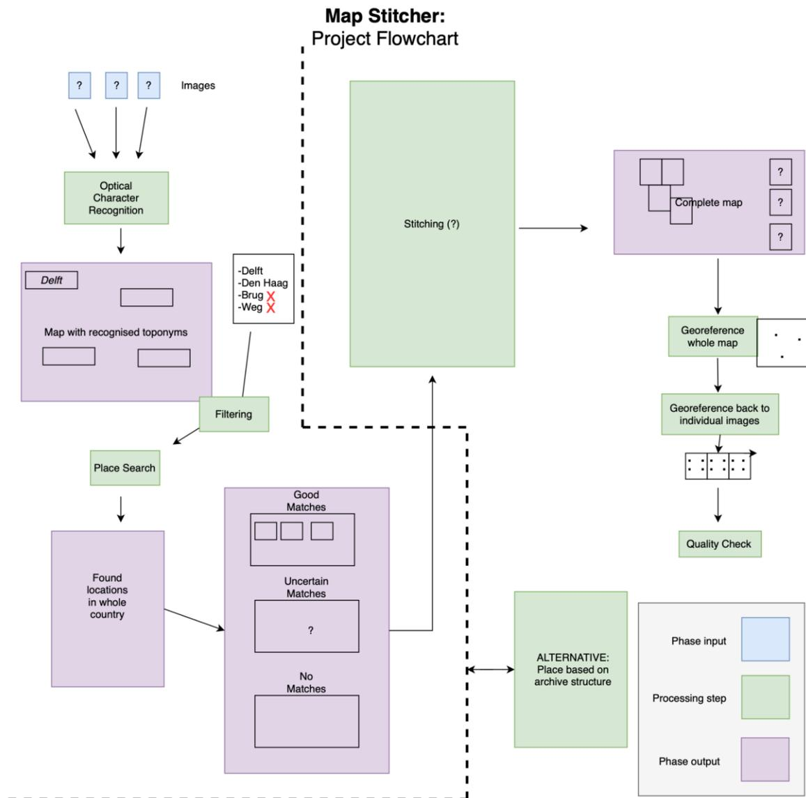
*Sketch flowchart of the map stitcher method. Starting from the top left, following the arrows it goes through a toponym searching phase (with as an alternative an archive structure method), a stitching phase, and a georeference phase.*
