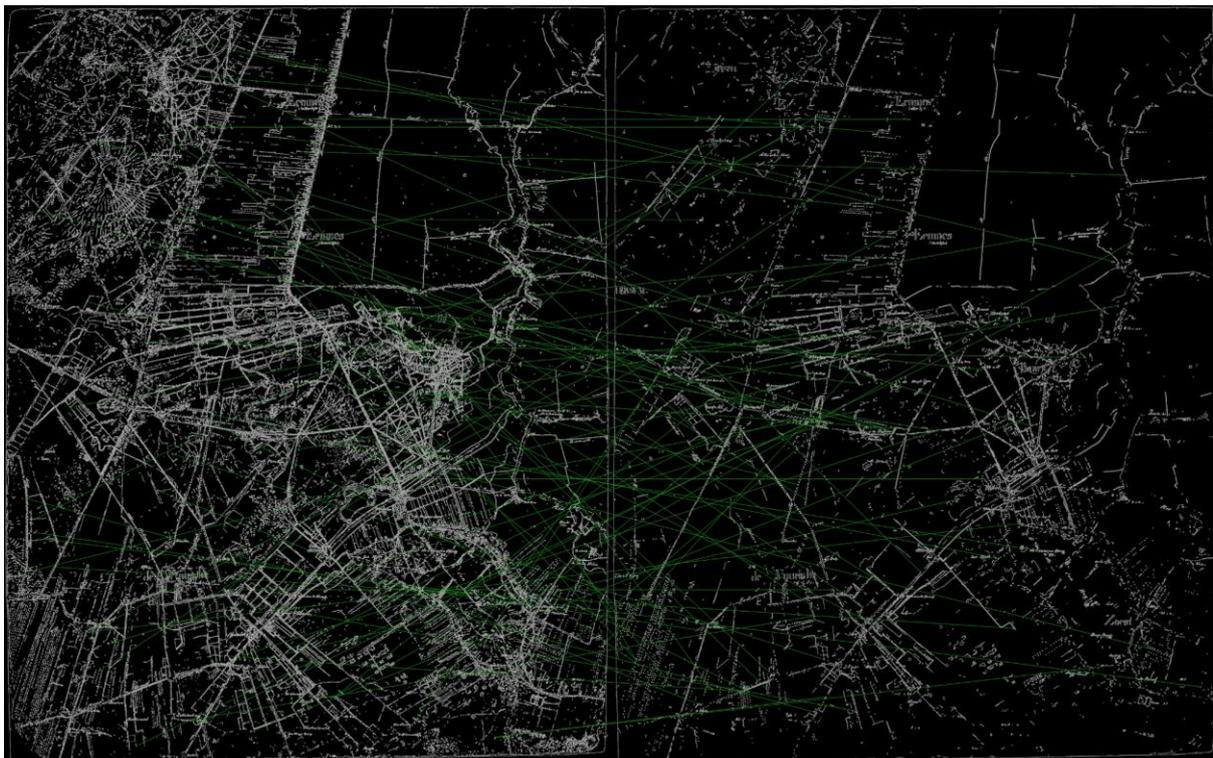
Figure 36 Subset of ORB feature detection match results on the same fieldminute (left and right) with altered edge detection parameters. Manual inspection revealed only one correct match.
