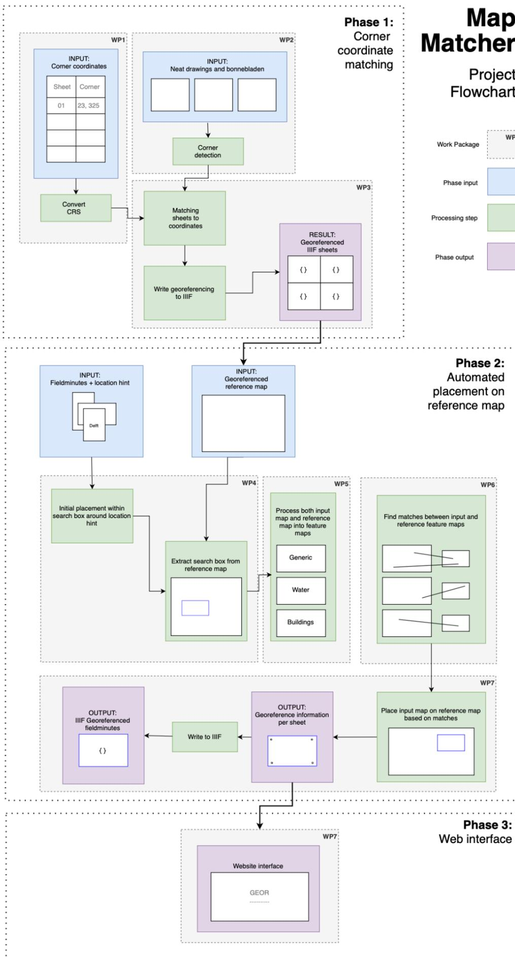
Figure 11 Sketch flowchart of the map matcher method. Starting from top left, following the arrows it goes through corner coordinate matching phase, an automated placement on reference map phase, and a web interface phase.
