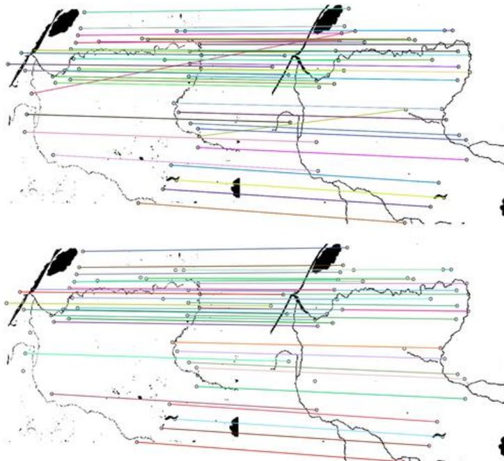
Figure 28 Result from Luft & Schiewe: Matches of detected features between source image (i.e., the segmented input map image, left) and the target image (i.e., the reference OpenStreetMap data, right). (Luft & Schiewe, 2021).
