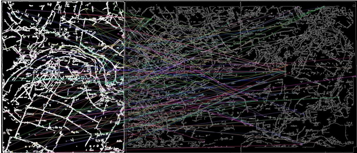
Figure 35 Subset from result from ORB based feature matching on edge masks of a fieldminute sheet (left) and a neatdrawing sheet (right).
