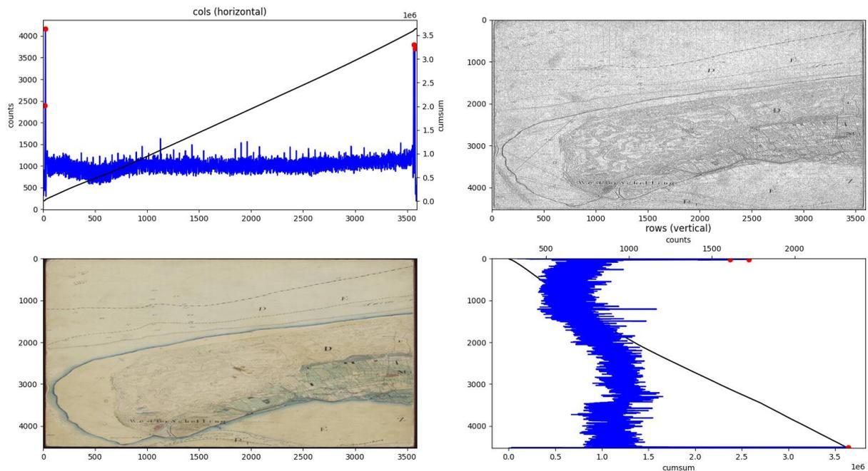
Figure 24 Example of identifying peaks of black pixels. The constant used is  $a=4$ . On top left is the number of black pixels per column. On top right the thresholded image. On the bottom left is the original image. On bottom right is the number of black pixels per row.
