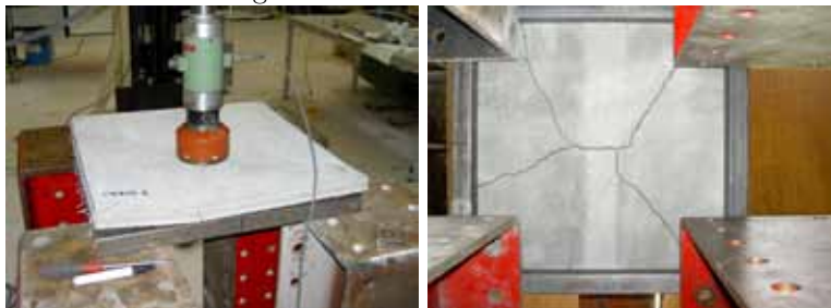
Figure 10.20: Crack develop on upper side of plate
