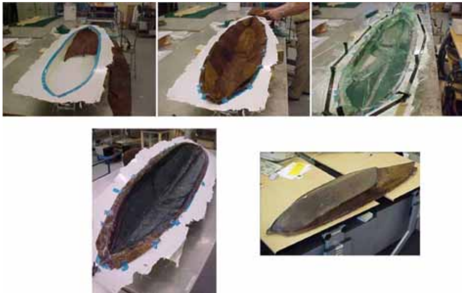
Figure 6.3: After the dry coir mats are placed into the mould, the material is bagged, the package is sucked vacuum and the resin is let in. The last pictures show the resulting product. [Brouwer et al., 2003]
