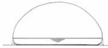
Figure 11.2: Closed formwork loaded with water, to reduce deformations at least 22 000 liter water is needed. Deformations at the sides are compensated with i.e. adobe before the ferrocement or concrete is applied.
