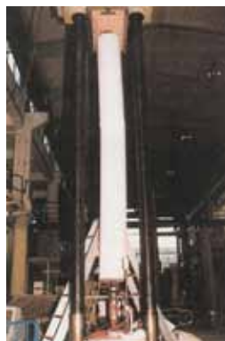
Figure 11.31: Results of the experiment of Frank Braam; a pneumatic tube loaded on pressure. The pneumatic tube has a span of 3 meter and a diameter of 30 cm [Braam, 2000].
