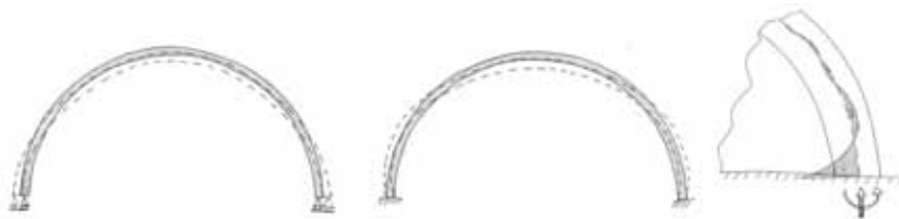
Figure 8.1: The connection to the foundation is rigid and prevents the shell from deforming as in most left sketch. Consequently the shell deforms as in the middle sketch. The moments that stem from this edge disturbance are shown in the sketch on the right.
