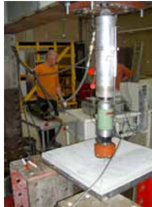
Figure 10.17: Testing a plate on concentrated load after two weeks of curing
