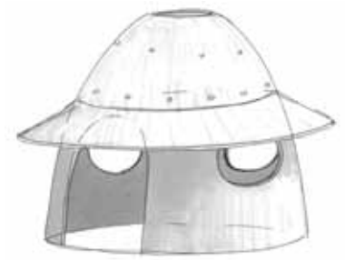
Figure 7.15: An example of a dome taking several of the matching building responses into account. However the hole in the roof should preferably be shaded by an elevated cover
