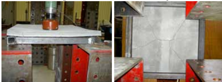
Figure 10.19: Growth of cracks
