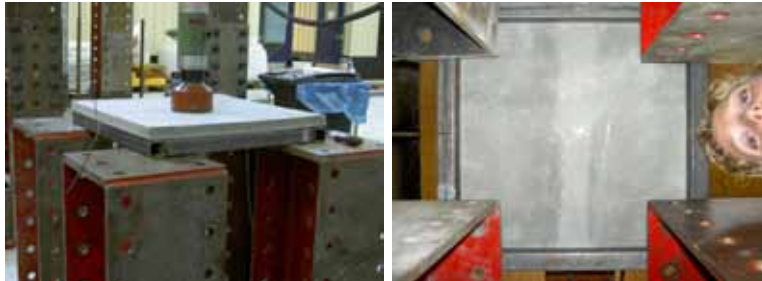
Figure 10.18: First cracks develop
