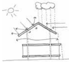
Figure 7.3: In these colonial bungalows in Singapore the most important function of the roof is to provide shade and protect the walls, allowing skin cooling through the use of lightweight materials. The large overhangs allow the windows to be left open in case of rain, allowing ventilations at all times except in storms. [Hyde, 2000]
