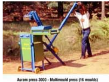
Figure 6.7: Press developed by the Auroville Earth Institute, India [Auroville, 2006]
