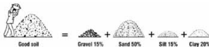
Figure 6.6: Proportions needed to produce CSEBs [Auroville, 2006]
