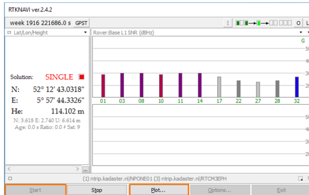
Figure 19. RTKNAVI operation window. Green light by the side of input stream indicates the software works properly.
