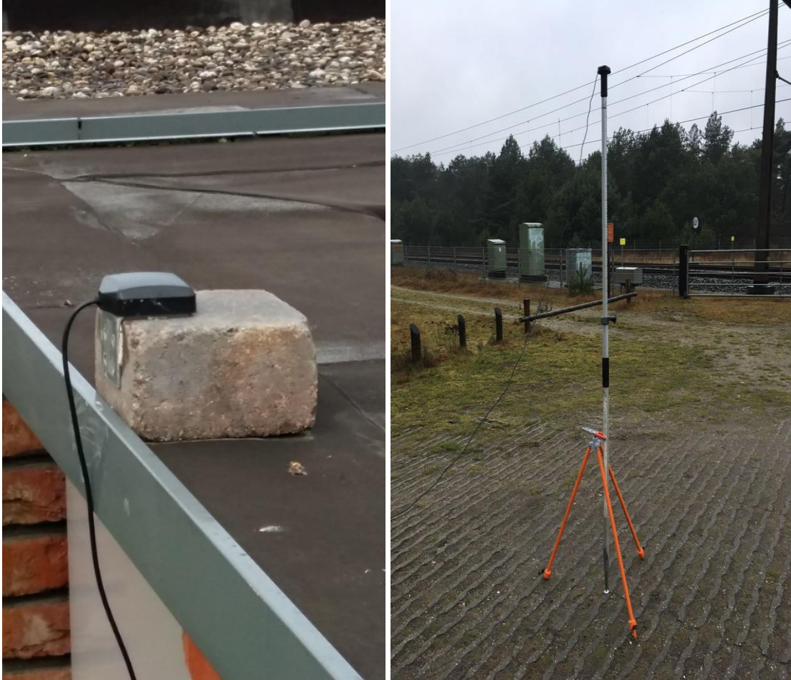
Figure 2. Base station (left) and rover setup of control point 1(right) pictures
