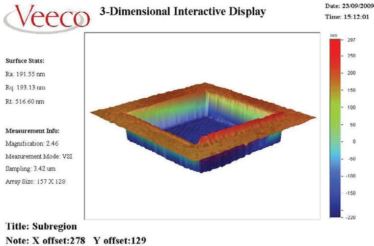
Fig. 6. 3D Profile of edge roughness of a  $350 \times 350 \mu\text{m}^2$  aperture after lift-off.
