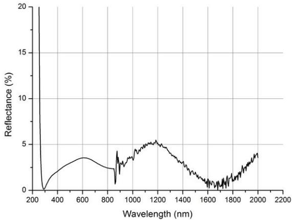
Fig. 4. Measured reflectance of the black coating
