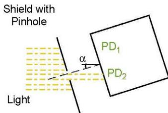
Fig. 2. Operation of the analog sun sensor
