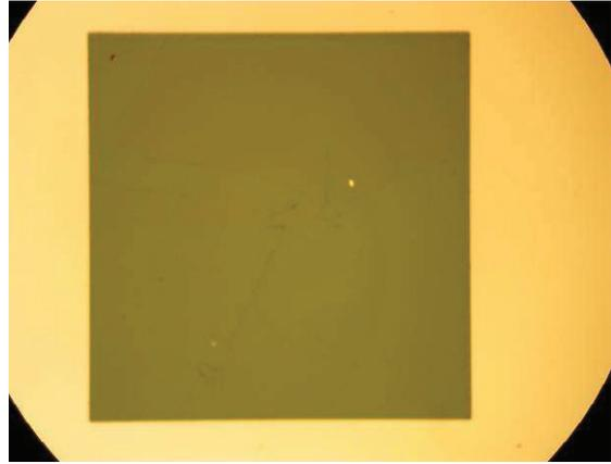
Fig. 5. Pinhole formation after lift-off processing.
