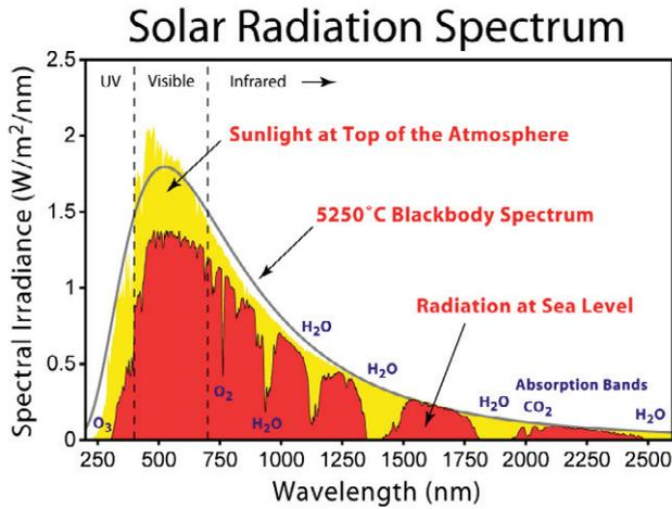
Fig. 1. Solar spectrum at the top of the atmosphere and at sea level [1]
