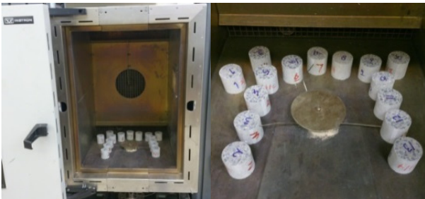
Figure 1: Concrete specimens in an environmental chamber.
