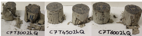
Figure 8: Failure mode of SCC concrete exposed to different fire temperatures and post-fire-cured for 7 days (2hr exposure time, quench cooling)
