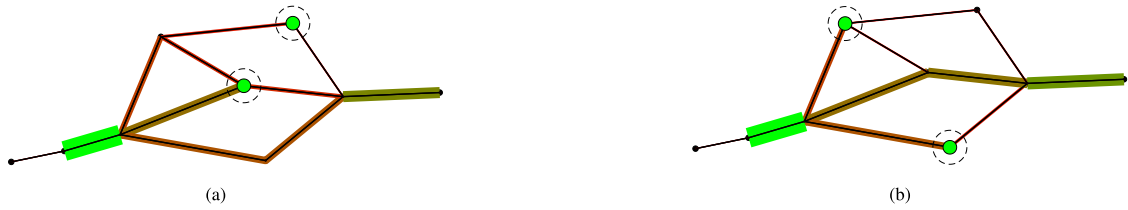
Fig. 3. The expected number of unobserved link arrivals, q^0(i|o, d) , for two different sensor configurations ( single-node construction) with a detection rate \theta = 0.7 . The wider and greener the link, the higher is the expected number of unobserved link arrivals. The most left link is defined as the origin and the most right link as the destination. The next-link probability matrix \mathbf{P}_d is based on link distances only plus a u-turn penalty. It can be seen that q^0(i|o, d) is practically zero for the origin link, since only link arrivals are counted.
