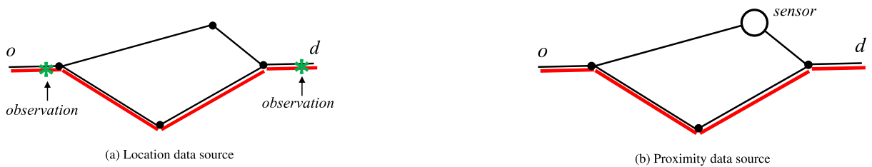
Fig. 1. Example showing the difference between (a) location data sources and (b) proximity data sources, with respect to route likelihood. In the case of location data it is impossible to distinguish from the two observations whether the individual took the upper or the lower (actual) route. In the case of proximity data, the absence of an observation of the individual near the sensor at the upper node makes the lower route much more likely to be the actual one.
