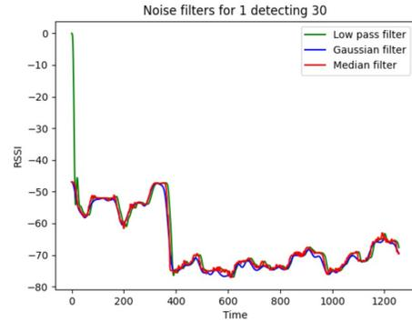
Figure 4: All 3 noise filters applied on the resulting RSSI signal from sensor 1 detecting sensor 30.
