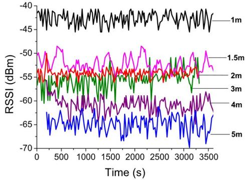
Figure 2: Distance measurements based on RSSI signals. Reprinted from [8].
