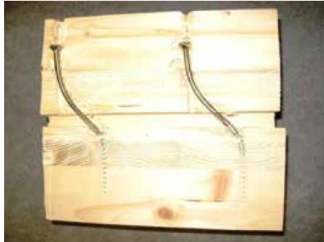
Fig 3.12 Ductile failure mode of metal connectors. (FPinnovations, 2013)
