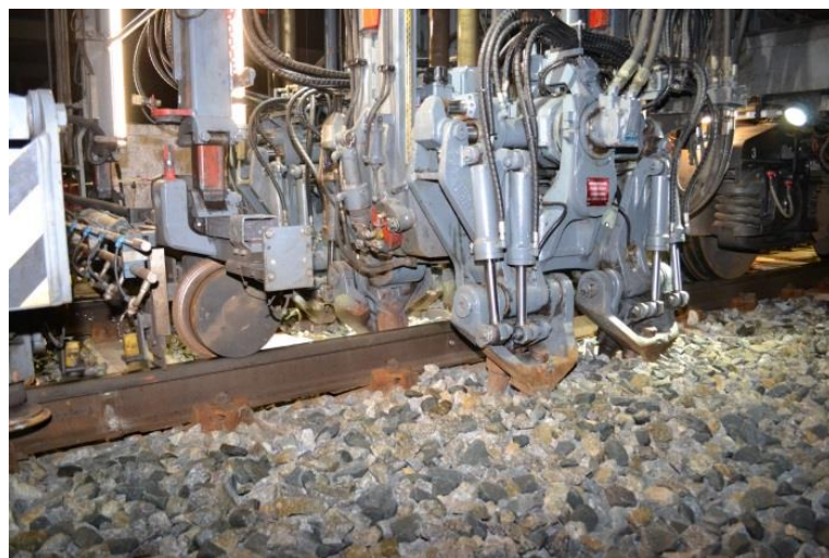
Figure 11. Tamping in a transition zone.
