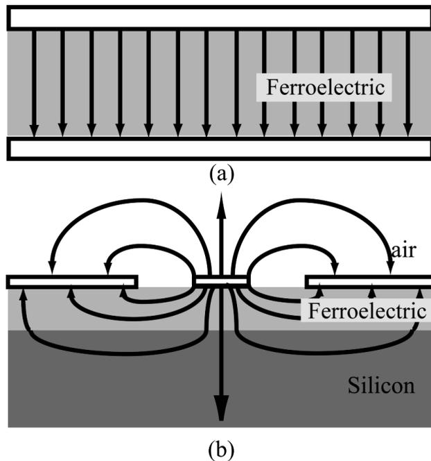
Figure 3.1 Schematic view of electric field distribution of a ferroelectric material based (a) parallel plate and (b) planar NDC varactor.
