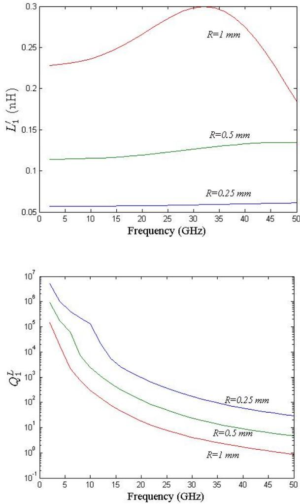
Figure 5.4: Equivalent inductance (left) and quality factor (right) of the lowest mode of the ADL disk resonator as a function of frequency for different values of the radius ( $R$ ). Simulations were carried out assuming a high-resistivity silicon substrate ( $\epsilon_s = 12$ ) with a thickness of 0.5 mm. No ground plane was assumed.
