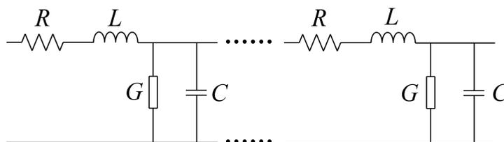
Figure E.1: Equivalent circuit model of a transmission line.  $L$ ,  $R$ ,  $C$  and  $G$  denote the series inductance, resistance and shunt capacitance, conductance (all per unit length), respectively.
