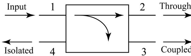
Figure 4.18: Schematic view of directional couplers and power flow conventions.
