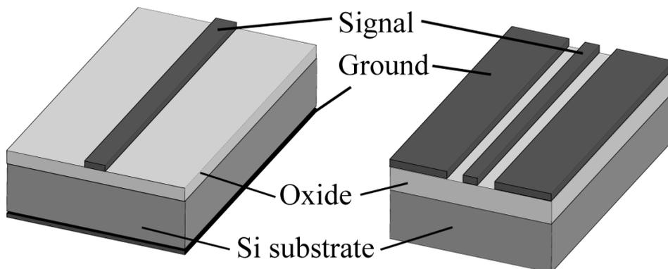
Figure 4.2 Schematic view of on-chip transmission lines with microstrip (left) configuration and coplanar-waveguide (CPW) configuration (right).
