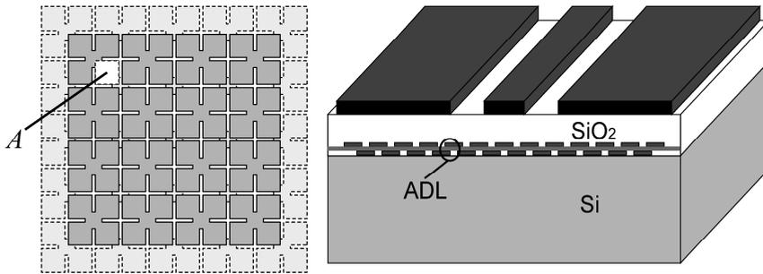
Figure 4.13: Top view (left) of a micro-patterned ADL. The micro-patterned ADL is realized by etching slots near the edges of each square pattern (dashed lines in the left figure). The schematic layout of an integrated CPW line equipped with an ADL shield is shown as well (right).
