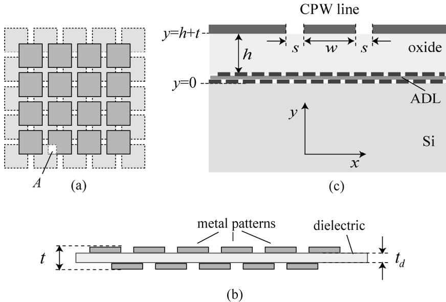
Figure 4.5 (a) and (b): Geometrical layout of the ADL consisting of two thin, patterned metal layers isolated by a thin dielectric. The lattices of squares on the two metal layers are shifted with respect to each other so that each square on the top lattice partially faces four squares on the bottom lattice and vice versa. (c): Cross section of an integrated CPW line shielded by an ADL inserted between the Si and oxide (thickness  $h$ ) layers.
