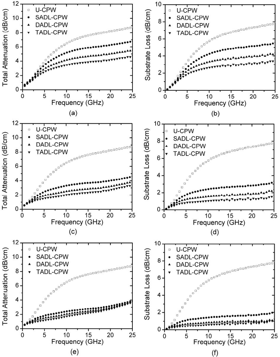
Figure 4.17: Extracted total attenuation (left column) and substrate loss (right column) for CPW lines ( $w=30 \mu\text{m}$ ,  $s=30 \mu\text{m}$ ) with different number of ADL shield layers. The ADL metal pattern sizes are  $3 \times 3$  (a-b),  $5 \times 5$  (c-d) and  $7 \times 7$  (e-f)  $\mu\text{m}^2$ .
