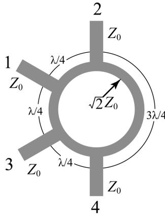
Figure 4.24: Geometry of a ring hybrid in microstrip form. Power entered at port 1 are equally distributed to port 2 and 3, with no power coupled to port 4.
