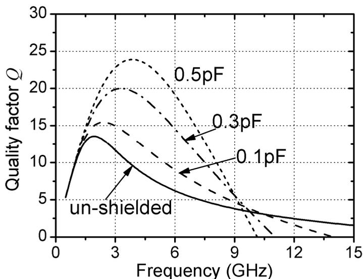
Figure 4.29: Simulated quality factor of a 1.5nH spiral inductor as a function of frequency with different values of  $C_{ADL}$ .
