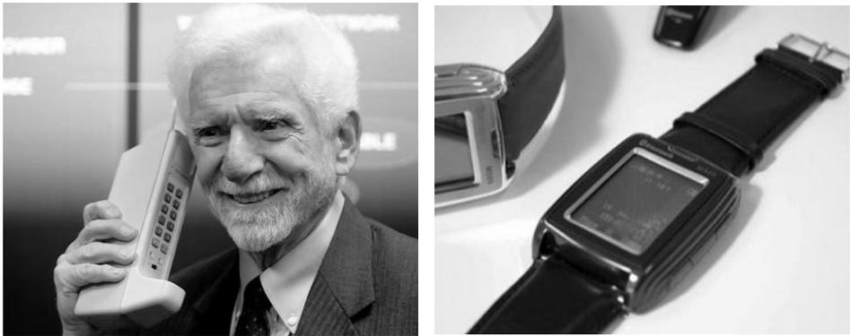
Figure 1.1: One of world's first cell phones held by inventor Martin Cooper, as compared to the wrist watch mobile phone packing a 1.5-inch touchscreen with tiny built-in stylus, bluetooth 2.0, MP4 and MP3 players.
