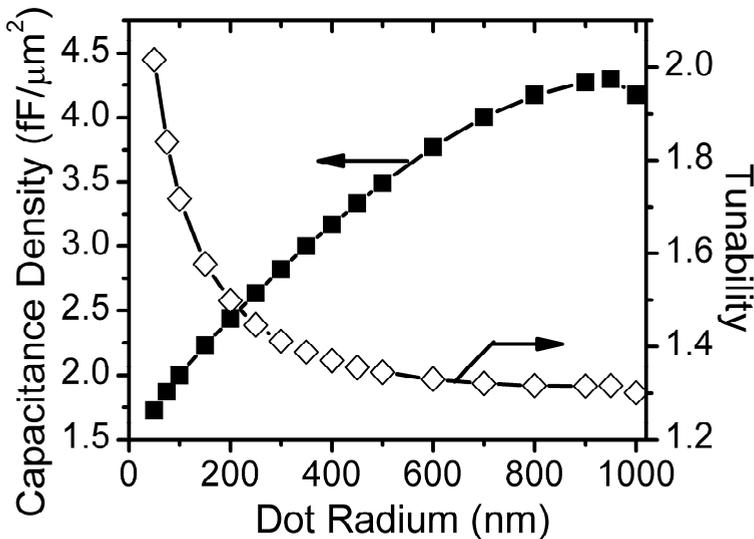
Figure 3.8: Calculated capacitance density (at zero voltage) and tuning factor (at 15 V) of a NDC array as function of dot radius. The BST and  $\text{SiO}_2$  layers were both  $1 \mu\text{m}$ -thick, and the inter-dot separation was  $2l = 2 \mu\text{m}$  in the calculations. A curvature of 30 nm was assumed at the bottom corner of the metallic dot to prevent the electric field exceeding the break down field of the BST ferroelectric.
