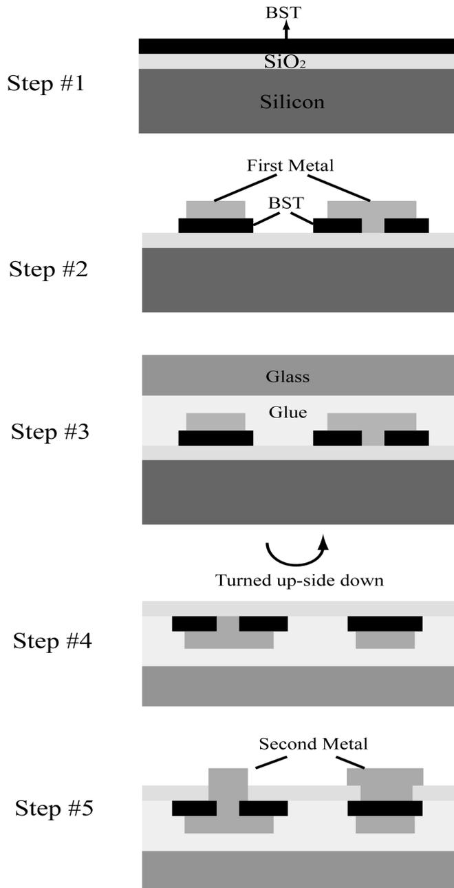
Figure 2.8 Sketch of STT process flow of ferroelectric tunable devices.
