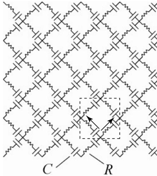
Figure 4.6 Network theoretical model of the ADL based on identical capacitors  $C$  and resistors  $R$ .
