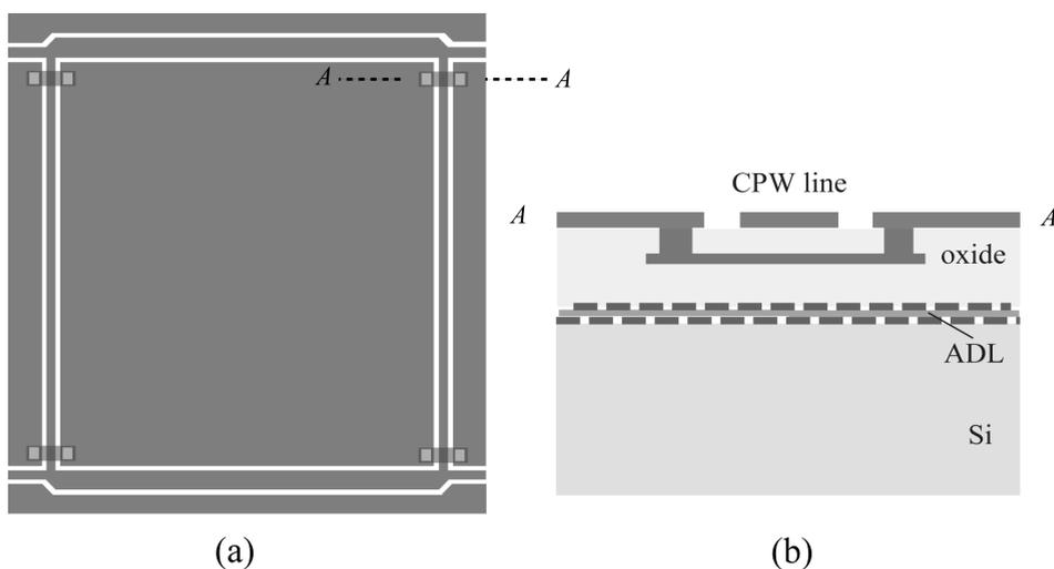
Figure 4.21: Schematic top view (a) and cross section view (b) of directional coupler with CPW configuration.
