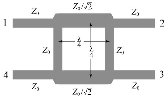
Figure 4.19: Geometry of a branch-line coupler in microstrip form. Power entered at port 1 are equally distributed to port 2 and 3, with no power coupled to port 4.
