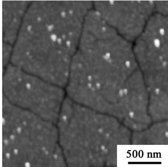
Figure 2.10: AFM image of BST thin film surface after STT processing shows micro cracks.
