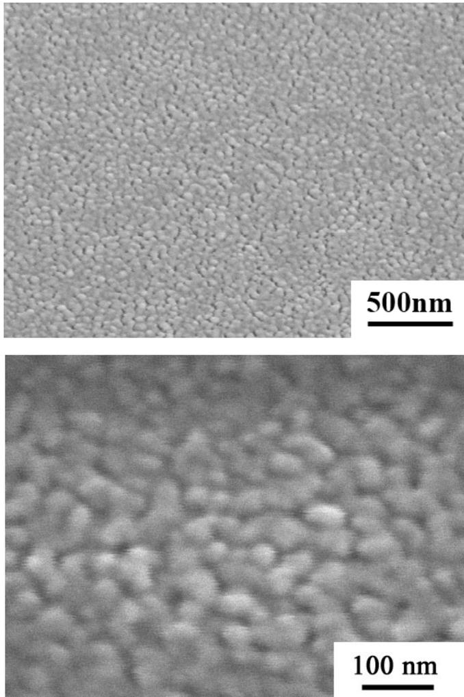
Figure 2.2: SEM images of  $\sim 40$  nm BST thin films by CSD method. The film is dense and without crack and fine grain size (30-50 nm) is clearly demonstrated.
