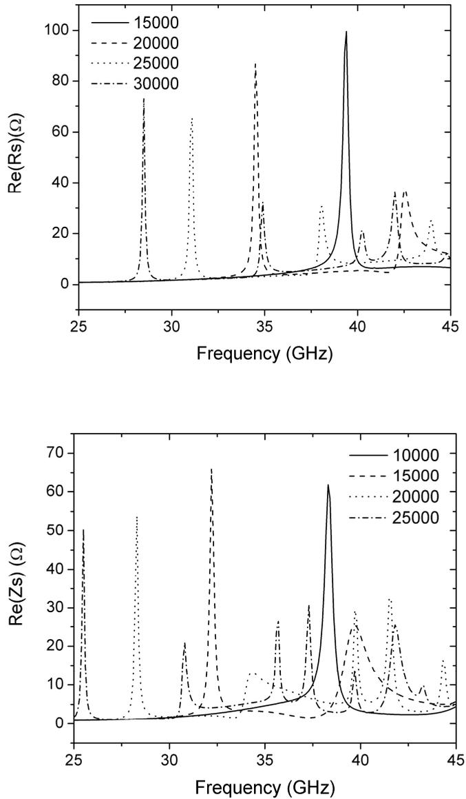
Figure 5.14: HFSS simulation results for ADL resonators of  $R=0.5$  mm (top) and  $R=0.75$  mm (bottom) with different values of in-plane effective dielectric constants, coupled with a dipole structure.
