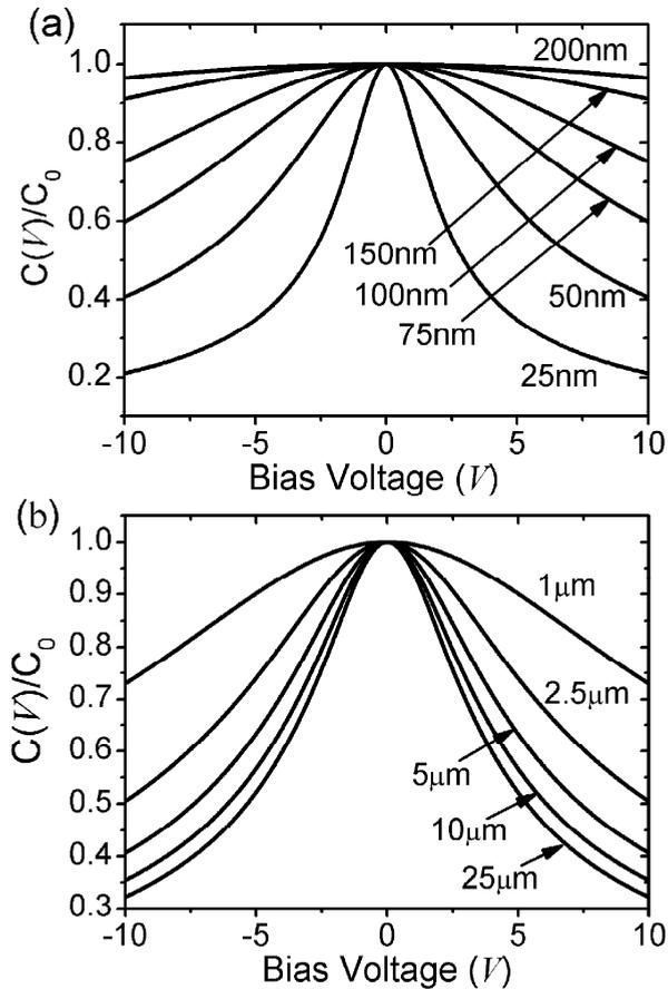
Figure 3.3: Calculated  $C$ - $V$  curves of a planar NDC varactor: (a) as function of the dot radius ( $R_d$ ) for a ferroelectric film thickness of  $5\ \mu\text{m}$ , and (b) as function of the ferroelectric film thickness ( $t_F$ ) for a dot radius of  $50\ \text{nm}$ .
