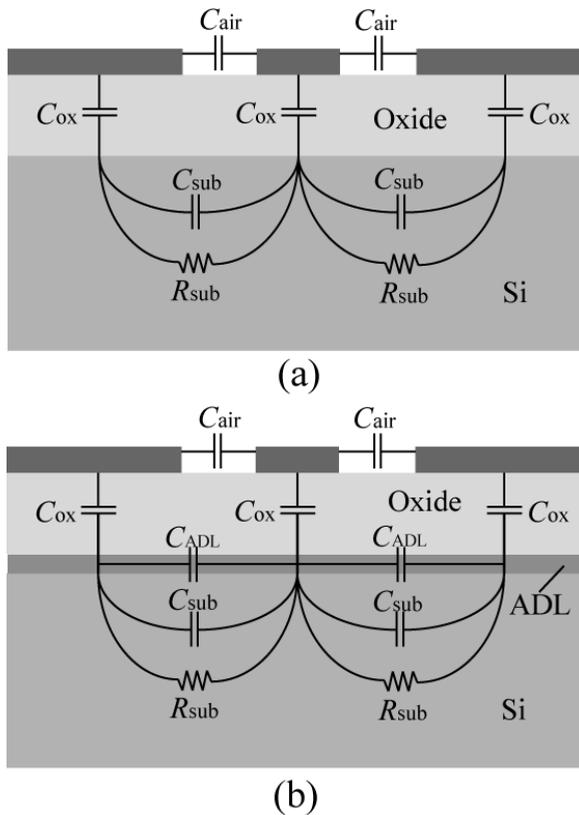
Figure 4.11: Cross section view and simplified lumped-element models of a CPW line on silicon with (a) and without (b) ADL shield.
