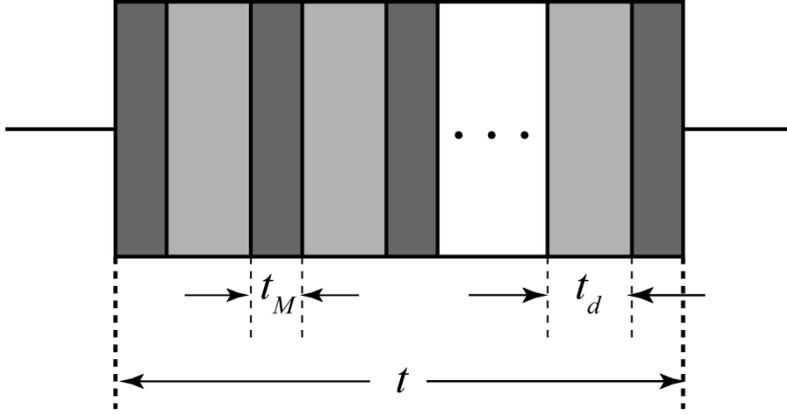
Figure 4.7: A simple model to calculate the perpendicular effective dielectric constant of general ADL structure.
