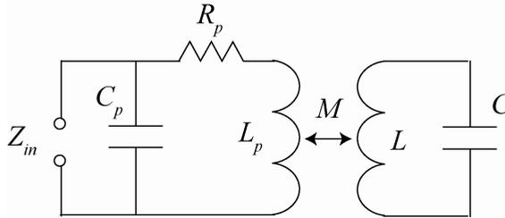
Figure 5.9: Equivalent circuit of the ADL resonator including a shunt capacitance  $C_p$ .
