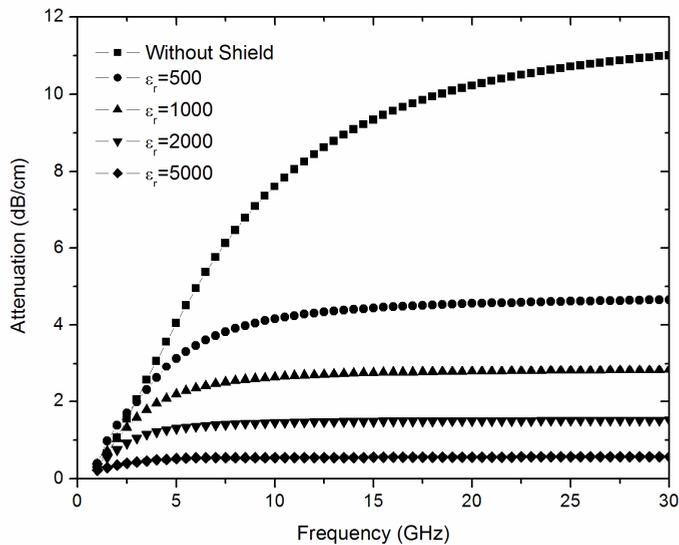
Figure 4.4: ADS Simulation results of CPW line attenuation as a function of frequency with super-k thin film shield for different dielectric constant values. For comparison, CPW line attenuation without shield is also shown.
