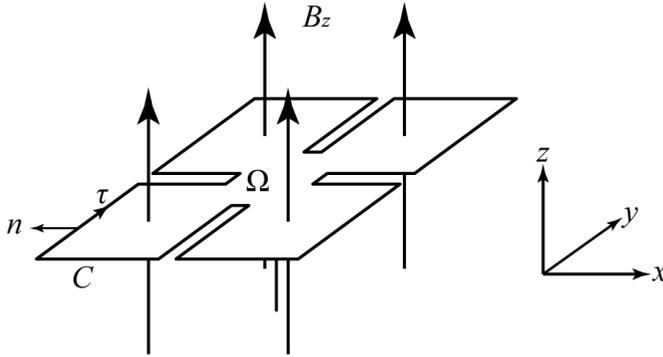
Figure C.1 A single ADL pattern under normal magnetic field. Also the coordinate system is shown.
