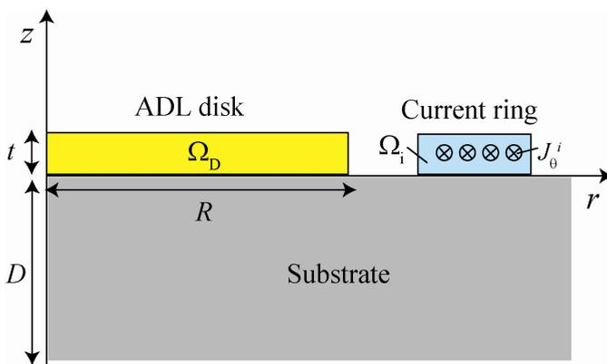
Figure 5.2: Cross section of the system in the  $r$ - $z$  plane. The cross section of the ADL disk and the current-carrying ring are denoted by  $\Omega_D$  and  $\Omega_i$ , respectively.
