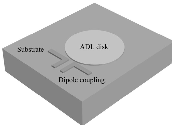
Figure 5.13: Schematic view of a weakly coupled ADL disk resonator, i.e., coupled with a dipole structure.
