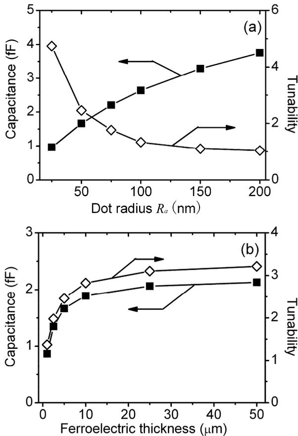
Figure 3.4: Calculated capacitance and tunability of a planar NDC varactor on silicon (a) as function of the dot radius ( $R_d$ ) for a ferroelectric film thickness of  $5 \mu\text{m}$ , and (b) as function of the ferroelectric film thickness ( $t_F$ ) for a dot radius of  $50 \text{ nm}$ . The applied dc bias voltage was  $10 \text{ V}$  in both cases.
