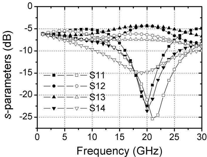
Figure 4.22: Simulated magnitudes of  $s$ -parameters (in dB) of CPW branch-line couplers on Si with (solid markers) and without (hollow markers) ADL shields.
