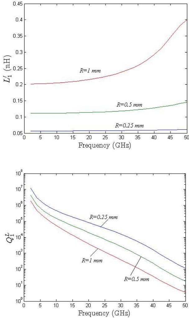
Figure 5.5: Equivalent inductance (left) and quality factor (right) of the lowest mode of the ADL disk resonator as a function of frequency for different values of the radius ( $R$ ). Simulations were carried out assuming a grounded high-resistivity silicon substrate with a thickness of 0.5mm. The thickness of the ADL disk was 1  $\mu\text{m}$ .
