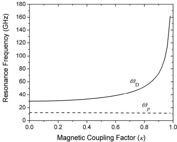
Figure 5.12: Calculated resonance frequency shifts as a function of magnetic coupling factor. Assume the ADL disk and the ring inductor have a first resonance frequency of 30 GHz and 12 GHz respectively.
