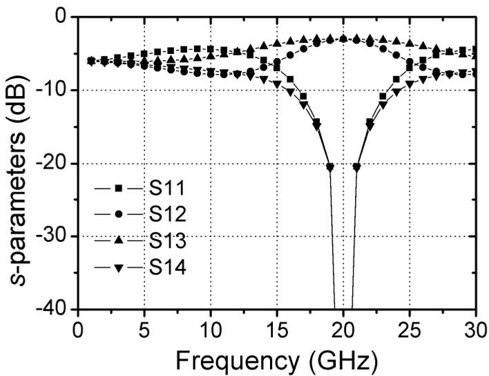
Figure 4.20: Magnitudes of  $s$ -parameters (in dB) of an ideal branch-line coupler as a function of frequency.
