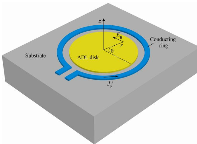
Figure 5.1: schematic of the ADL disk resonator. A conductive, current-carrying ring encloses a thin disk of artificial dielectric with the radius  $R$ . The ring and the disk are placed on top of a substrate which is assumed to be unbounded in the horizontal plane. The current flowing through the ring is considered as an impressed source, inducing an electromagnetic field with the components  $E_\theta, H_r, H_z$  in the system.
