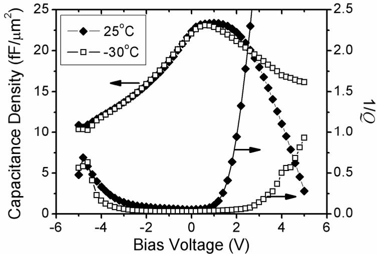
Figure 2.6: Capacitance density and capacitor losses of Al/BST/Pt thin film varactor as a function of applied bias voltage on Pt electrode.
