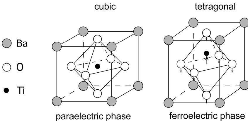
Figure 1.4: Crystal structure of BaTiO<sub>3</sub> for a cubic paraelectric phase without spontaneous polarization and a tetragonal ferroelectric phase with spontaneous polarization along [001] direction.
