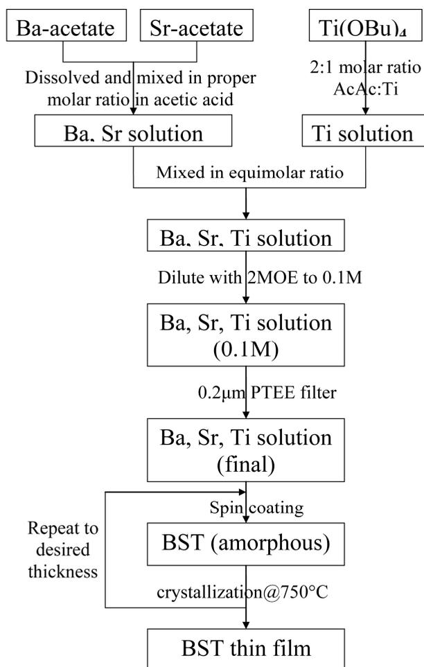
Figure 2.1: Process flow of BST thin film preparation by CSD method.
