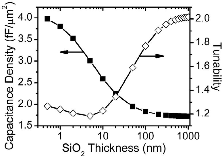
Figure 3.10: Calculated capacitance density (at zero voltage) and tuning factor (at 15 V) of a NDC array as function of the SiO<sub>2</sub> layer thickness. The BST layer was 1 μm-thick, the dot radius was 50 nm, and the inter-dot separation was  $2l = 2 \mu\text{m}$  in the calculations.
