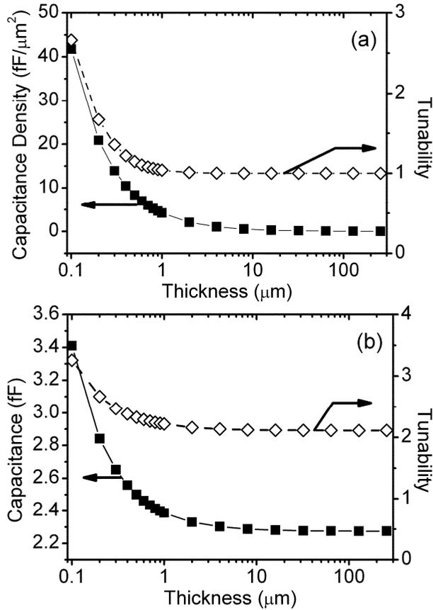
Figure 3.5: Calculated capacitance and tunability vs. ferroelectric material thickness for (a) a parallel plate capacitor and (b) a NDC capacitor built from a metallic dot (radius 50 nm) placed above a grounded ferroelectric layer. The applied dc bias voltage was 5 V in both cases.
