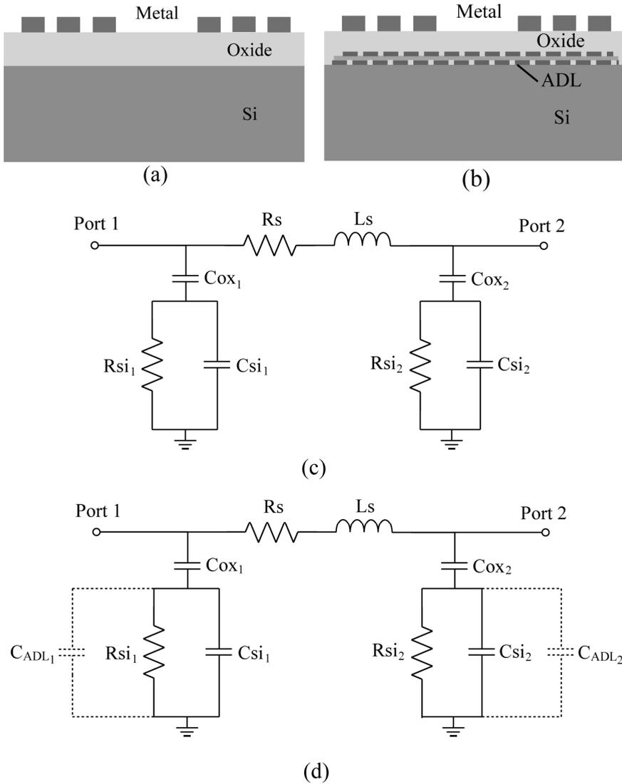
Figure 4.28: Cross section views of spiral inductors (a) on Si substrate without ADL shields and (b) with ADL shields. Also shown simplified equivalent lumped element models of spiral inductors (c) on Si substrate without ADL shields and (d) with ADL shields.
