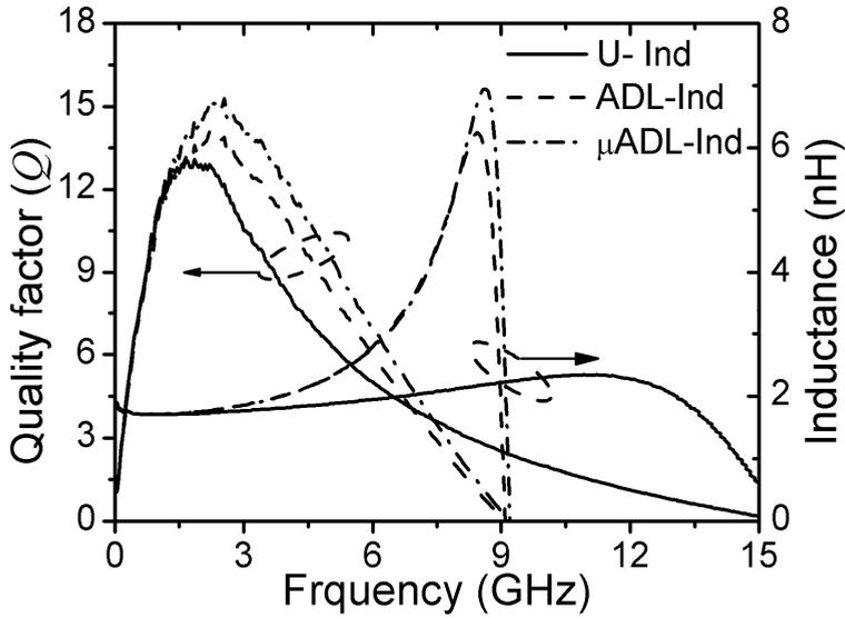
Figure 4.30: Measured quality factor and inductance value of a 2nH spiral inductor as a function of frequency with ordinary (ADL-Ind) and micro-patterned ( $\mu$ ADL-Ind) ADL shields. Results for un-shielded spiral inductor (U-Ind) are shown as well for comparison.
