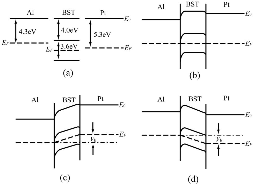
Figure 2.7: Band diagrams of Al/BST/Pt capacitor, (a) the work functions of Al and Pt, the electron affinity and band gap of BST; (b) band diagram of Al/BST/Pt when contacts are formed and equilibrium is established; (c) band diagram of Al/BST/Pt when negative bias voltage is applied at Pt; (d) band diagram of Al/BST/Pt when positive bias voltage is applied at Pt.
