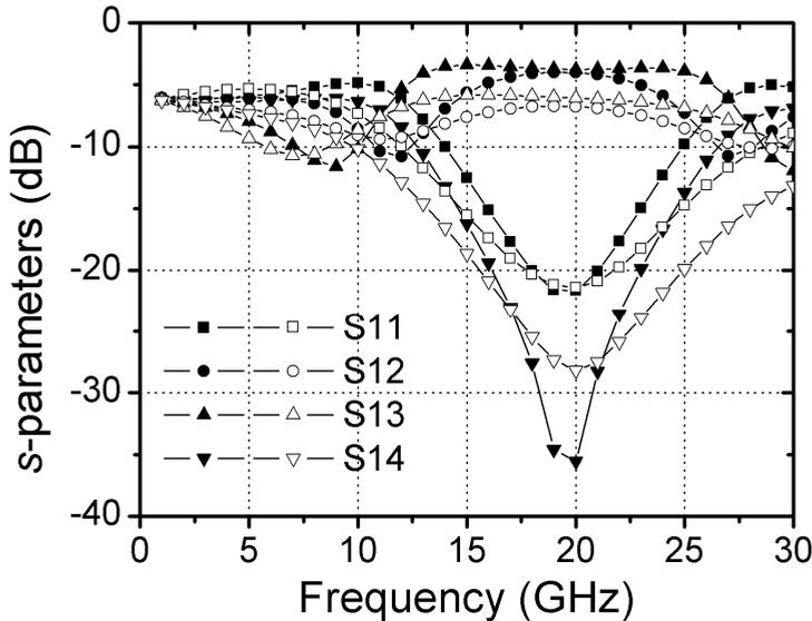
Figure 4.27: Simulated magnitudes of  $s$ -parameters (in dB) of CPW ring hybrids on Si with (solid markers) and without (hollow markers) ADL shields as a function of frequency.
