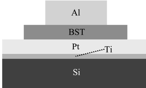
Figure 2.4: Cross section view of of Al/BST/Pt thin film varactor.
