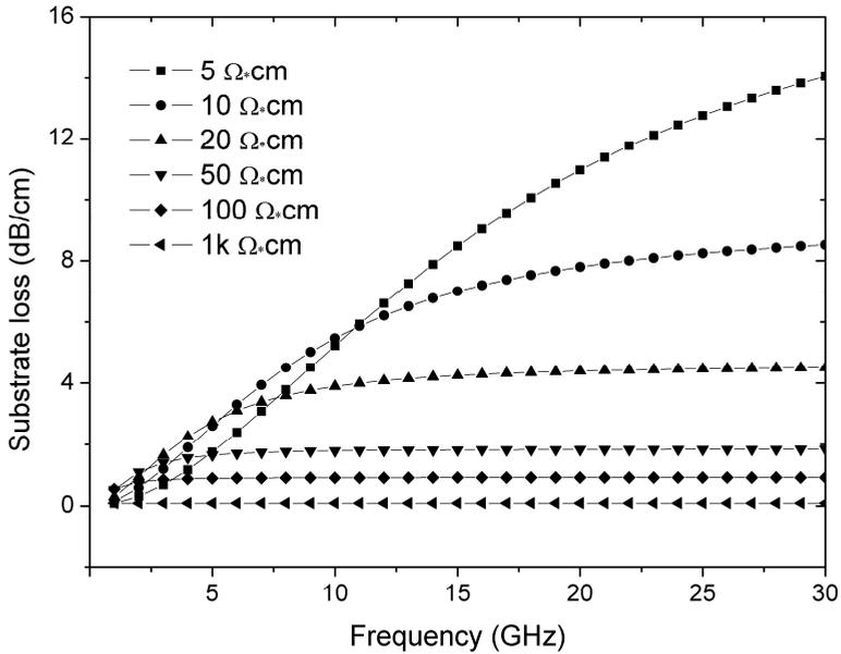
Figure 4.1: ADS Simulation results of CPW line attenuation as a function of frequency for different substrate resistivity.
