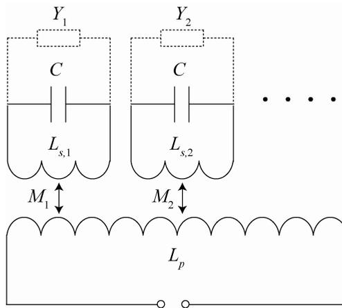
Figure 5.3: Equivalent circuit of an ADL disk resonator. Note that, in general, all the component values are complex and frequency dependent.
