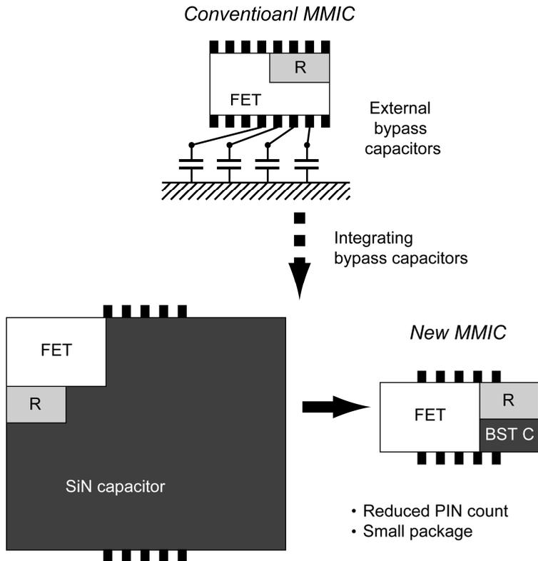
Figure 1.5: Area comparison of MMIC in case of using SiN and BST capacitors. Adapted from [43].
