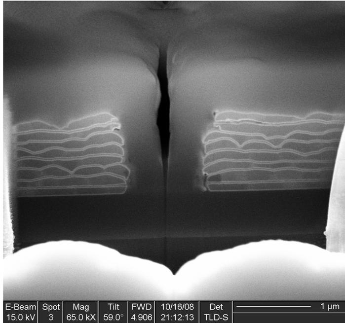
Figure 5.16: SEM image of cross section of ADL resonator. Eight layers of the metallic patterns in ADL are resolved. The local narrowing of the metallic layer is also shown.
