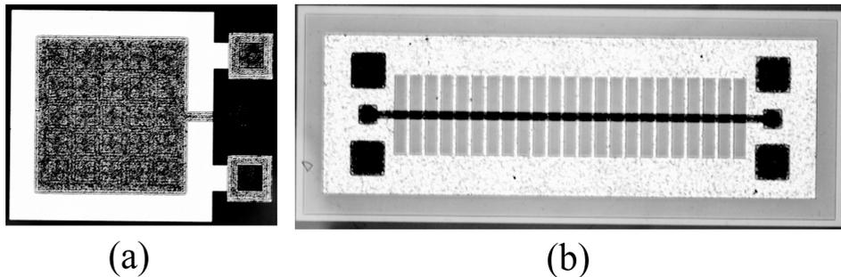
Figure 2.9: Micrographs of as-fabricated (a) parallel plate varactor and (b) microstrip transmission line.
