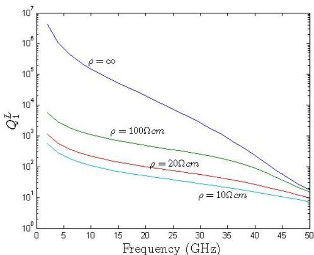
Figure 5.6: Inductive quality factor of the first mode of an ADL disk (radius 0.5 mm, thickness  $1 \mu\text{m}$ ) on a silicon substrate (0.5 mm-thick, with a ground plane) as function of frequency for different values of substrate resistivity  $\rho$ .
