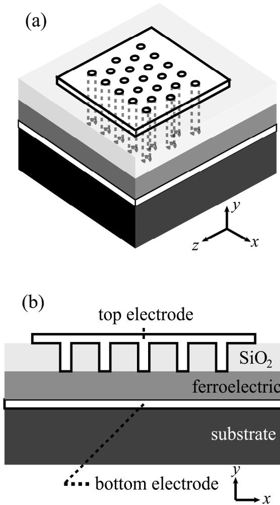
Figure 3.6: (a) 3D and (b) cross section view of arrayed NDC varactor.
