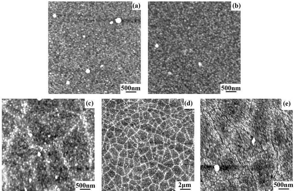
Figure 2.11: AFM images of surface morphologies of BST thin film after (a) 3 times, (b) 6 times, (c) 9 times coating-crystallization cycles; (d) large area scan of 9 layers shows network of bright line segments; (e) the line segments were identified to be micro-cracks after wet etching in 0.55HF solution.
