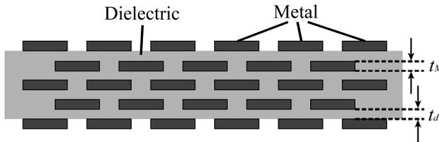
Figure 4.16: Cross section view of multi-layered ADL.
