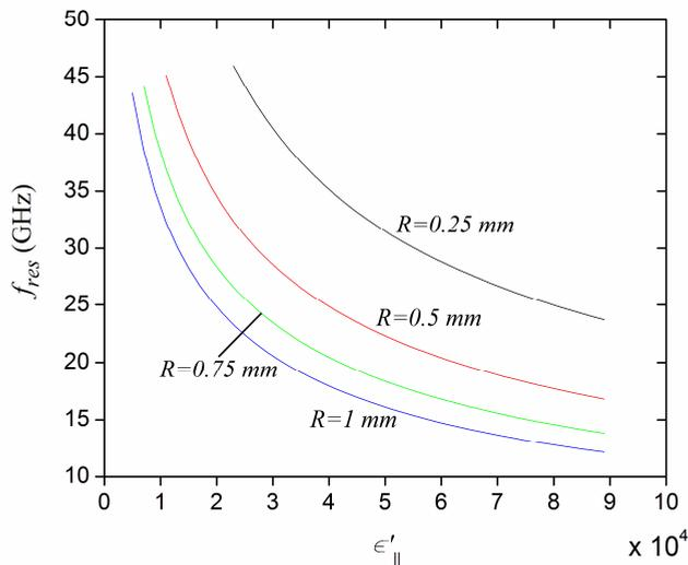
Figure 5.11: Resonance frequency of the first mode of the ADL disk as function of the in-plane dielectric constant for different disk radii. A grounded AF45 glass substrate with a thickness of 0.7 mm was assumed. The ADL thickness was 1  $\mu\text{m}$ .
