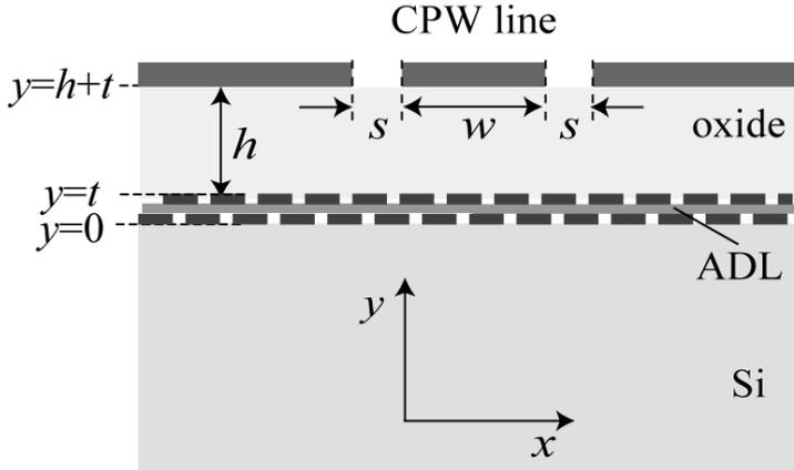
Figure D.1 Geometrical layout of CPW with ADL shield. The thickness of the ADL and oxide are  $t$  and  $h$  respectively.
