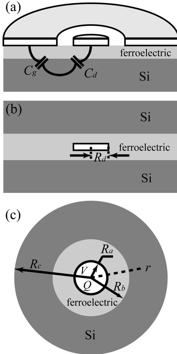
Figure 3.2: (a) Schematic view and simplified equivalent lumped element model of a planar NDC varactor; (b) Self capacitance of the NDC varactor is simplified to a system with a dot sandwiched between two identical ferroelectric/silicon substrate; (c) The system in (b) is further mapped to a spherical model for semi-analytical analysis.
