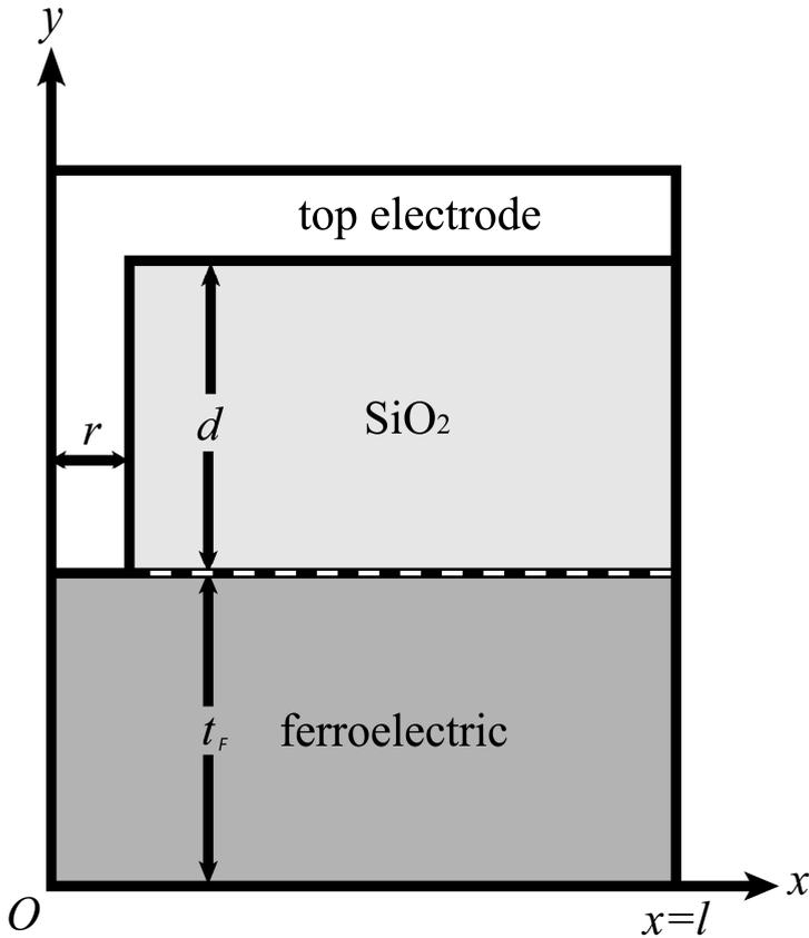
Figure 3.7: Cross section geometry of a unit cell (only right half is shown) of arrayed NDC varactor.
