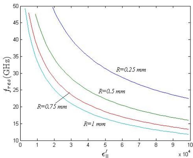
Figure 5.7: Resonance frequency of the first mode of the ADL disk as function of the in-plane dielectric constant  $\epsilon'_{||}$  for different disk radii. A grounded high-resistivity silicon substrate with a thickness of 0.5mm was assumed. The ADL thickness was  $1 \mu\text{m}$ .
