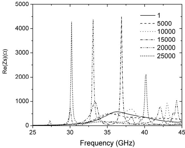
Figure 5.10: HFSS simulation results for ADL disk resonators ( $R=0.75$  mm) with different values of in-plane effective dielectric constants, coupled with ring inductor.
