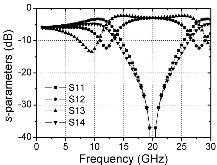
Figure 4.25: Magnitudes of  $s$ -parameters (in dB) of an ideal ring hybrid as a function of frequency.
