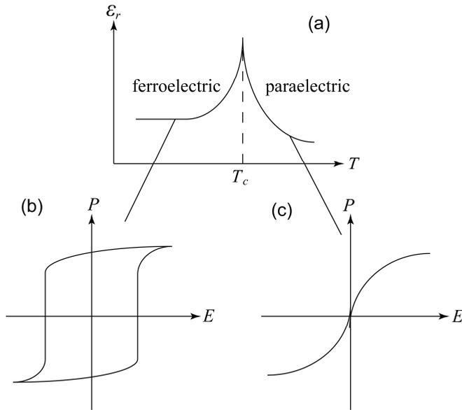
Figure 1.3: Schematics of (a) relative dielectric constant as a function of temperature in different phases; (b) hysteresis loop of polarization-electric field in a ferroelectric phase and (c) nonlinear polarization-electric field relation in a paraelectric phase.
