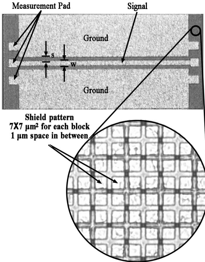
Figure 4.8: Micrograph of a CPW transmission line with an ADL substrate shield. The signal line width and signal to ground spacing of the CPW are denoted by  $w$  and  $s$ , respectively. The enlarged portion of the ADL shield clearly shows the two (overlapping) metallic square lattices.
