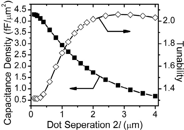
Figure 3.9: Calculated capacitance density (at zero voltage) and tuning factor (at 15V) of a NDC array as function of inter-dot separation. A BST and  $\text{SiO}_2$  layer thickness of  $1\mu\text{m}$ , and a dot radius of  $50\text{nm}$  were assumed in the calculations.
