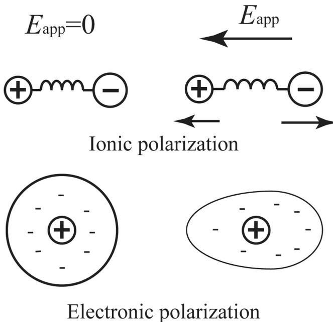
Figure 1.2: Schematics of ionic polarization and electronic polarization.
