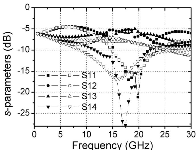
Figure 4.23: Measured magnitudes of  $s$ -parameters (in dB) of CPW branch-line couplers on Si with (solid markers) and without (hollow markers) ADL shields.
