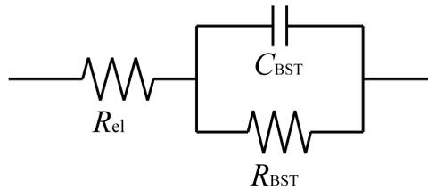
Figure 2.5: Equivalent circuit model of BST thin film capacitor.
