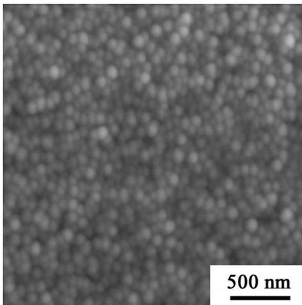
Figure 2.3: Surface morphology of 150 nm BST thin film by AFM. Smooth surface is identified.
