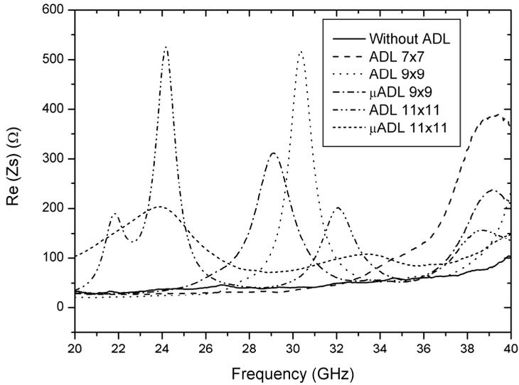
Figure 5.15: Measurement results for ADL resonators ( $R=0.75$  mm) with different ADL patterns.
