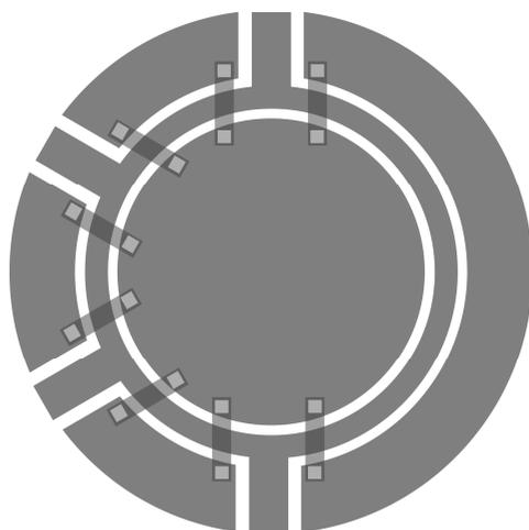
Figure 4.26: Schematic top view of the layout of a ring hybrid in CPW form. Additional metal bridge under the CPW layer is added and connected to CPW grounds by through dielectric vias.
