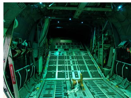
(a) Cargo bay with attachment points along the fuselage length (attachment points shown in red). (b) Back door of the cargo bay of the inspected military cargo aircraft.
