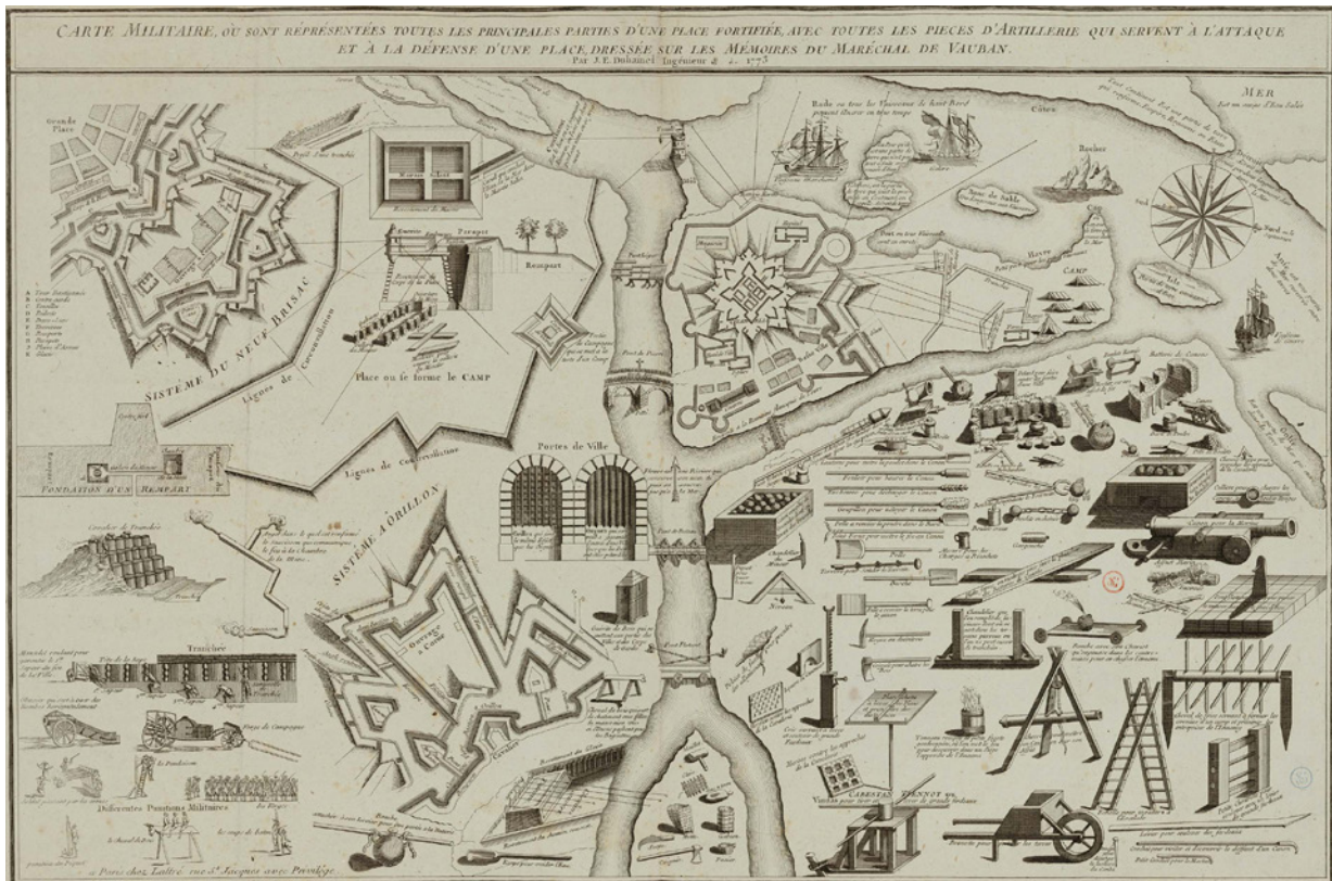
Fig 5.10 Design principles for fortifications Drawn against a hypothetical background, the map presents Vauban's design principles and the main components of fortifications as well as the equipment needed to destroy them. Mantiene claims this map was still available in Vietnam in 1921, along with Vietnamese translations for the different parts depicted. J.E. Duhamel (1773), Carte militaire, où sont représentées les principales parties d'une place fortifiée , Paris : Chez Latrappé.
