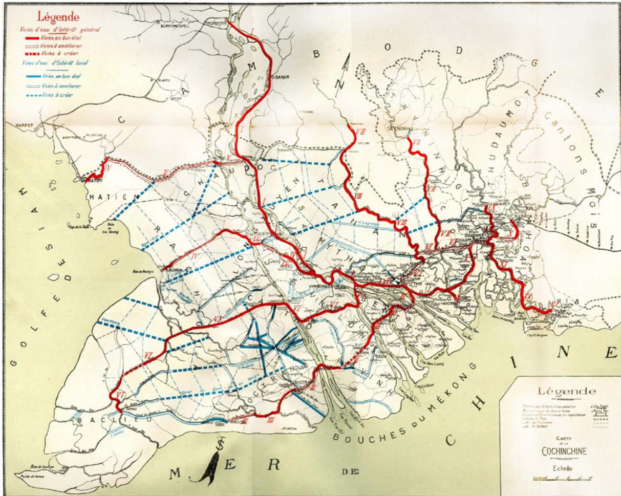
Fig 6.2 Waterway network Drawn by Albert Pouyanne who would subsequently become Chief Engineer of public works in the colony, the map shows the relationship between regional (red) and local (blue) waterways. Proposed canals (dotted lines) are arranged to intersect at regular intervals and appear to extend to the limits of the colony's jurisdiction. Albert Pouyanne (cartographer) (1911), Voies d'eau de la Cochinchine , Saigon: Impri. nouvelle.
