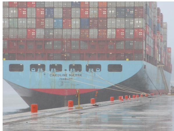
Figure C.5: Mooring configuration of the Caroline Maersk. The photo shows the stern of the vessel, where 4 breast lines and 2 spring lines are visible. (Own photo, 29 Sept. 2018)
