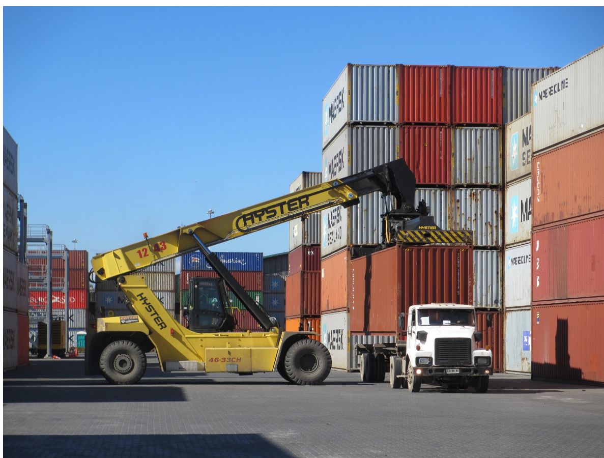
Figure 6.1: A reach stacker is loading a tractor in the storage area. The container is transported towards the quay where it will be loaded on the container vessel
