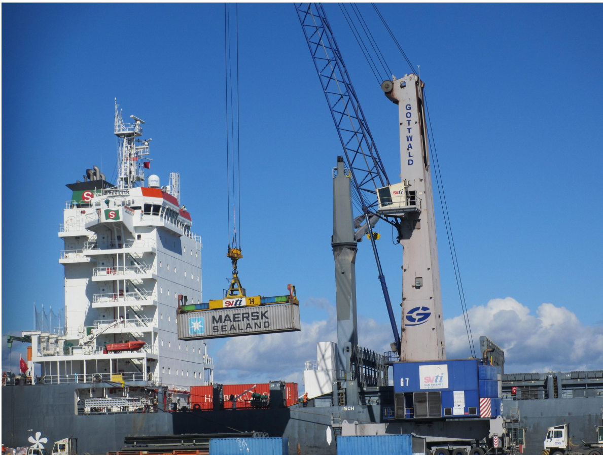
Figure 9.1: Unloading of a container vessel by mobile cranes
