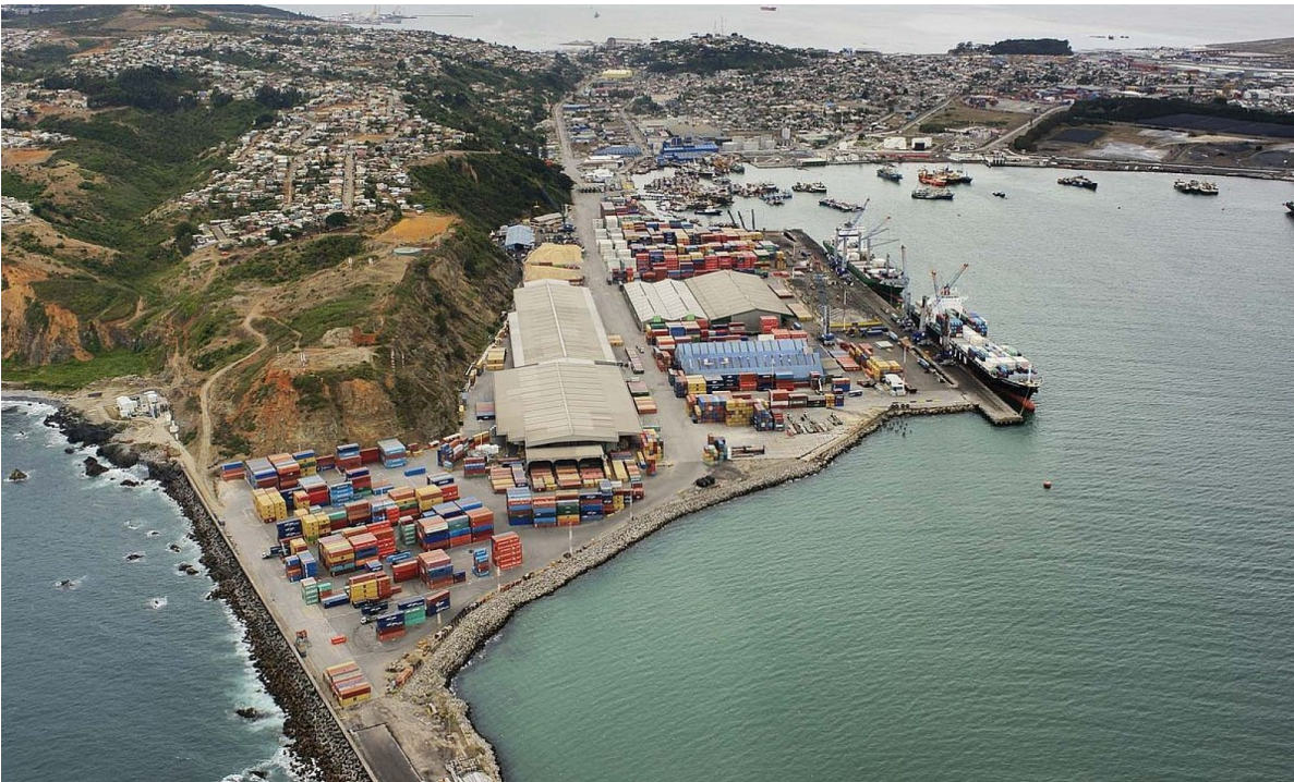
Figure 2.1: Historical (2006) aerial view of the San Vicente Port. The port consists of a multipurpose terminal. The quay has been extended so that the terminal now has 5 berths. Also, new warehouses have been constructed and old ones have been removed.
