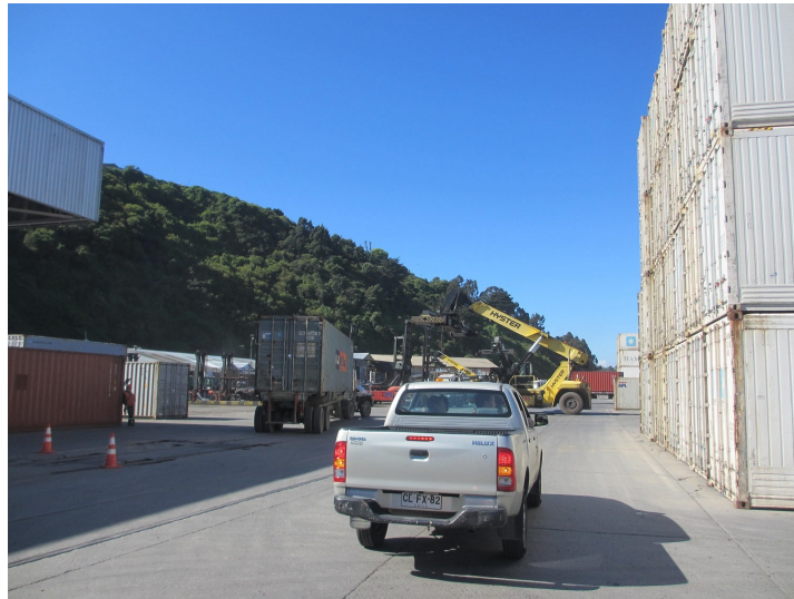
Figure D.5: Congestion in the main road due to Reach Stacker operation. The Reach Stacker will pick up the grey container from the trailer and place it in the area behind the warehouse (in the left of the figure). This process was observed during the site visit and took about 2 minutes.
