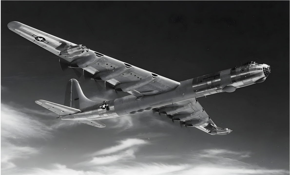
Figure 1.5: Convair B-36J-III “Peacemaker” military aircraft featuring multiple ram-air intakes located at the wing leading-edge for aerodynamic and cooling efficiency purposes.
