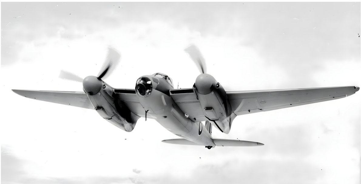
Figure 1.6: De Havilland Mosquito DH-98 military aircraft featuring two engine cooling ram-air ducts positioned in the inboard section of the wing.
