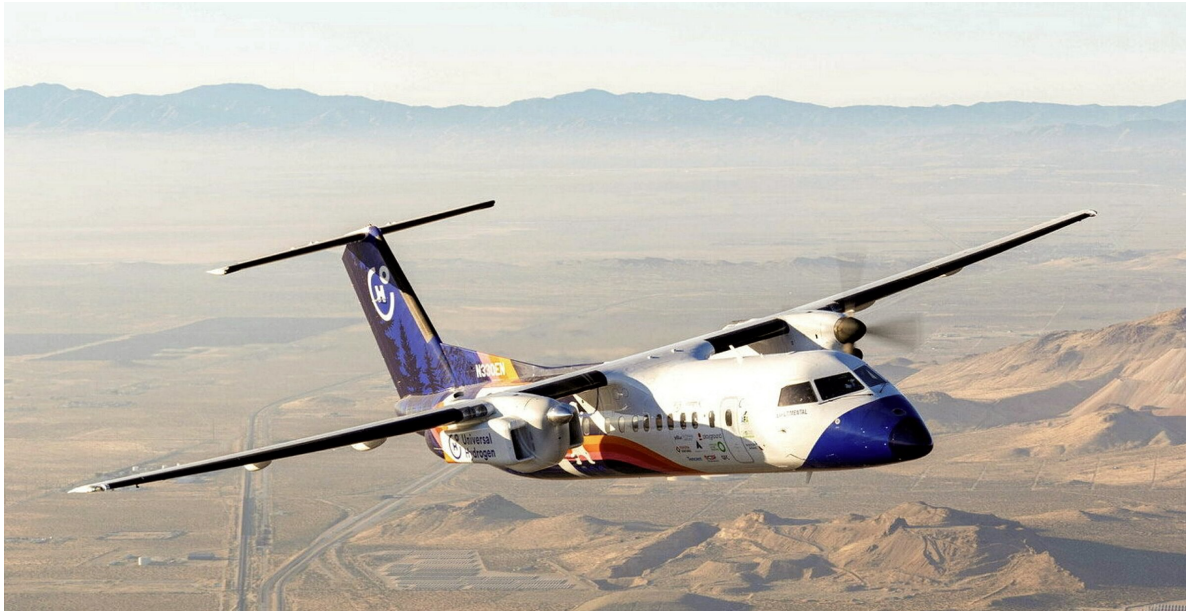
Figure 1.1: Universal Hydrogen's De Havilland Canada Dash-8, retrofitted with hydrogen fuel-cell technology. The turboprop engine on the starboard wing integrates prominent ram-air cooling ducts housing heat exchangers on both sides of the nacelle to manage the thermal demands of the FCS.
