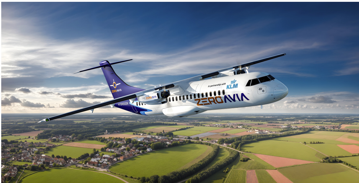
Figure 1.2: ZeroAvia's ATR-72, retrofitted with a hydrogen-electric powertrain. The nacelle features a four-duct ram-air configuration, each duct channeling airflow to different components to meet the cooling demands of the FCS. Image credit: ZeroAvia and KLM Royal Dutch Airlines.
