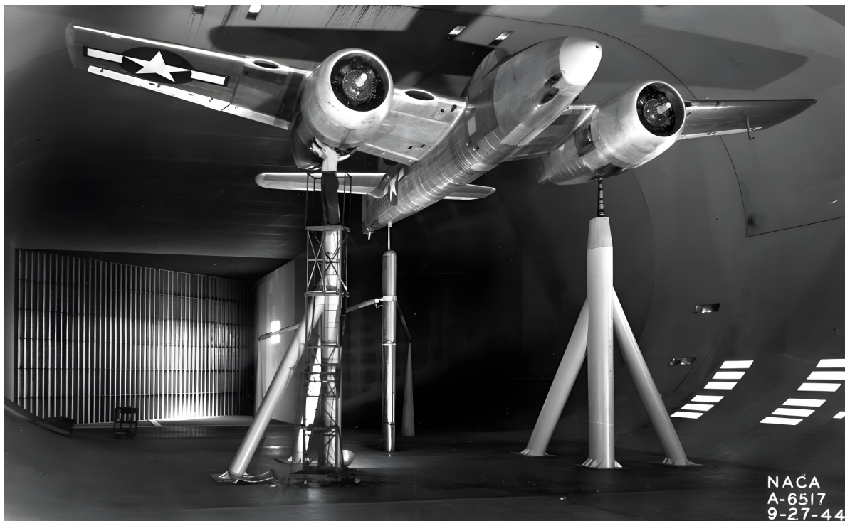
Figure 1.4: Grumman XF7F-1 Tigercat fighter aircraft, mounted in the Ames 40-by 80-foot wind tunnel to investigate wing-integrated duct performance under propeller slipstream effects [8].
