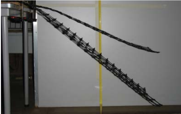
Figure 4.5: Difference in deflection due to the own-weight in longitudinal and transversal direction
