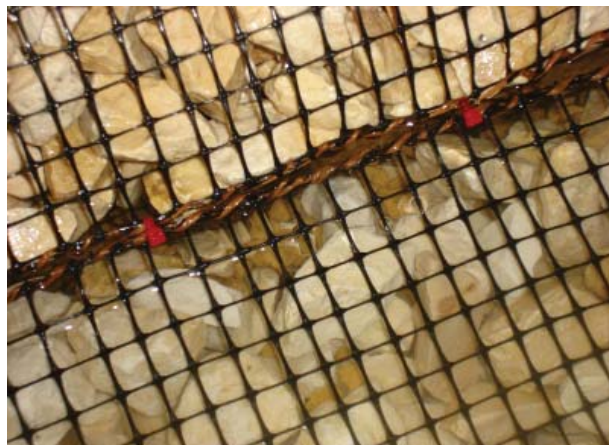
Figure 5.7: Experiment D6 too large fill material
