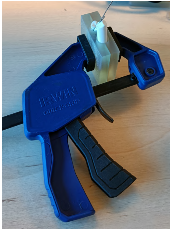
Figure B.1: Tube bending process where the tube has been heated with a heat gun and subsequently bent into shape and placed in the mould to cool. The silicon tube with attached wire can be seen still present within the tubing.
