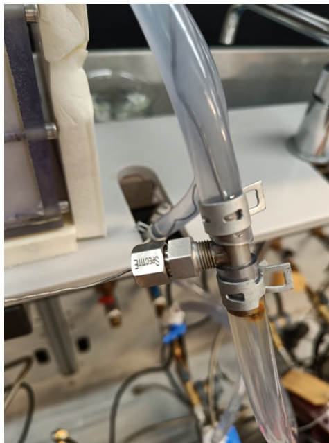
Figure B.16: Image of a welded thermocouple t-junction
