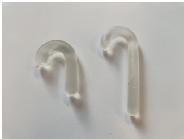
Figure B.2: Left: The first iteration bending tube with a shorter handle and larger tube diameter. Right: The second iteration bending tube with a larger handle, increased chamfer, and a smaller diameter.
