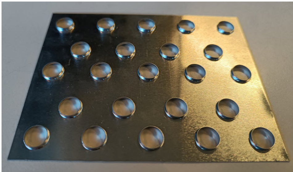
Figure B.5: Image of fins with pressed collars form optimal thermal contact.
