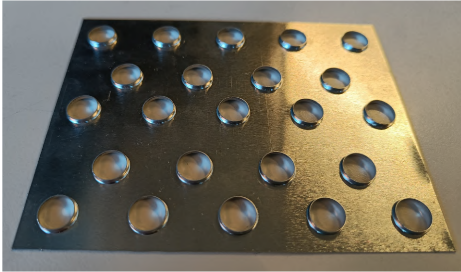
Figure 5.2: Single cooling fin
