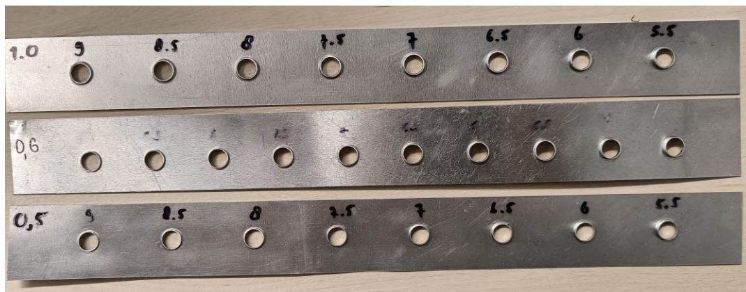
Figure 5.1: Test strips used to dimension the collars. The thicker fins were capable of producing higher collars before tearing. The thicker fins are less flexible.
