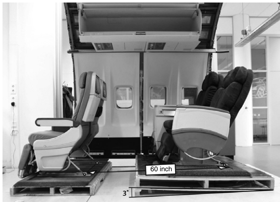
Fig. 2. Inclination angle and pitch length.
