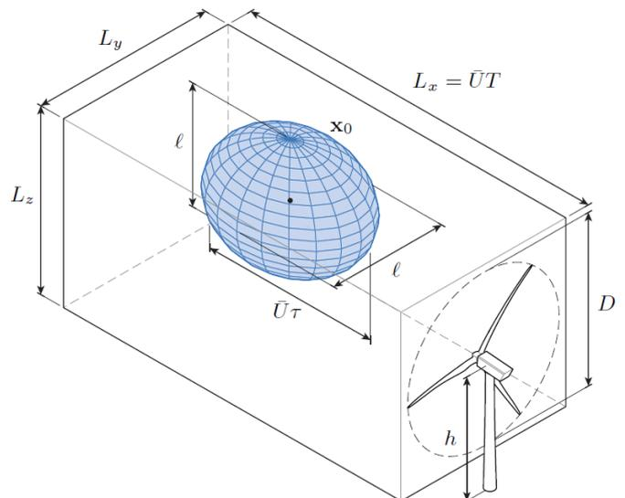
Fig. 1 Sketch of a gust in a constrained wind field, showing all the relevant parameters.
