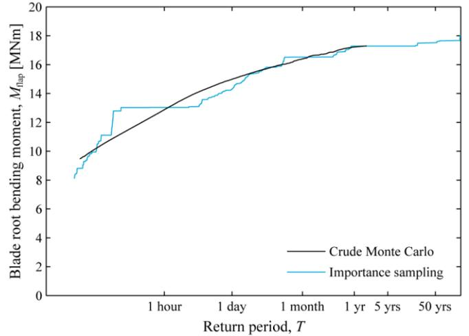
Fig. 6 Return level plot of the extreme blade root flapwise bending moments at  $18.5 \leq \bar{U} \leq 19.5$  m/s, constructed from a crude Monte Carlo simulation ( $N = 1 \cdot 10^5$ ) and an importance sampling method ( $N = 3 \cdot 10^3$ ).
