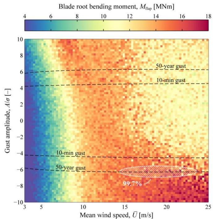
Fig. 3 Extreme blade root flapwise bending moments in response to a gust of amplitude  $A$  at a mean wind speed  $\bar{U}$ . The white hatched area marks 99.7% ( $\pm 3\sigma$ ) of the sample space.
