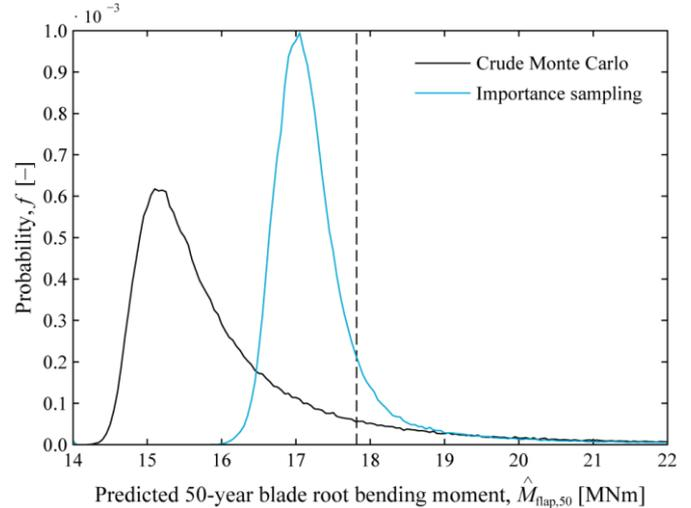
Fig. 7 The uncertainty in the predicted 50-year blade root flapwise bending moments based on 1 day of simulated time. Indicated with a dashed line is the “true” 50-year load based on 96 years of data (17.8 MNm).
