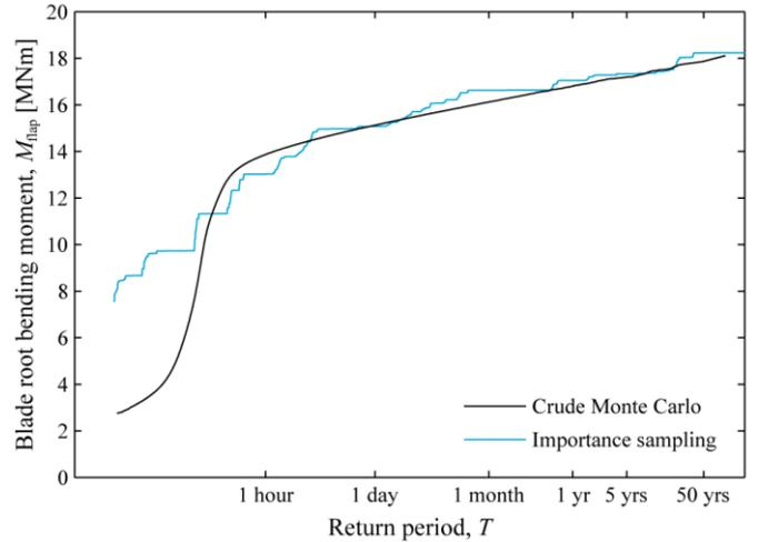
Fig. 5 Return level plot of the extreme blade root flapwise bending moments, constructed from a crude Monte Carlo simulation ( $N = 5 \cdot 10^6$ ) and an importance sampling method ( $N = 1 \cdot 10^5$ ).
