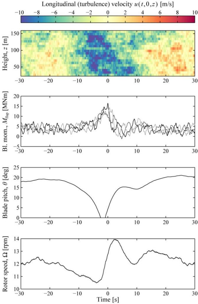
Fig. 4 An extract of a ten-minute time series at  $\bar{U} = 22$  m/s with an extreme blade root bending moment of 16.4 MNm.
