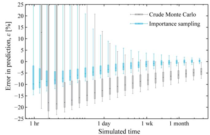
Fig. 8 Box plots showing the error in the prediction of the 50-year blade root flapwise bending moment for both methods. The thick line in the box represents the median, the edges of the box are located at the first and third quartile, and the ends of the whiskers mark the 5<sup>th</sup> and 95<sup>th</sup> percentiles.
