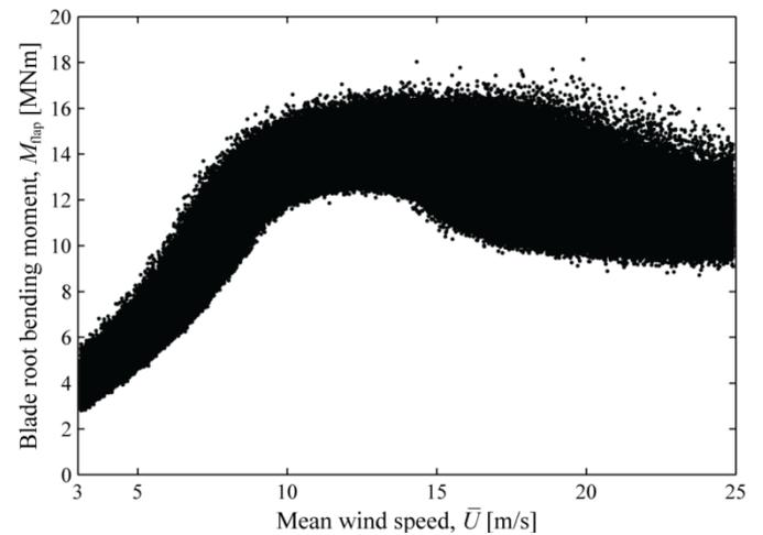
Fig. 2 Extreme blade root flapwise bending moments obtained from the reference data set, plotted as a function of the mean wind speed  $\bar{U}$ .
